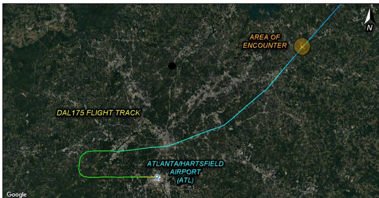
Figure 3. Overhead view of latter segment of the accident flight track of DAL175 with area of turbulence encounter highlighted, destination airport depicted, and overlaid onto satellite imagery.
