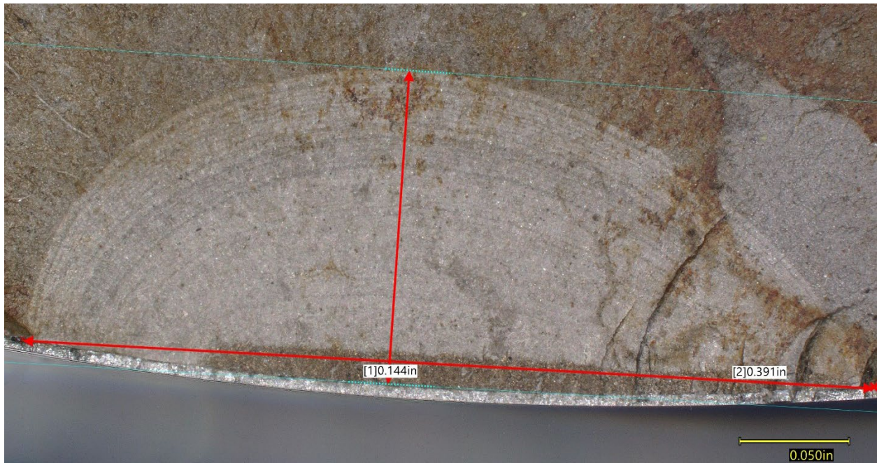
Figure 2. Microscopic view of the thumbnail crack in Figure 1., annotated to show various dimensions.
