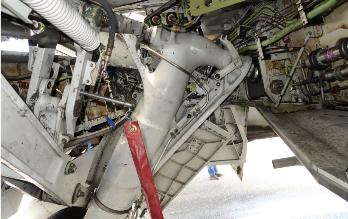
Figure 1. View of the fractured and damaged areas of the main landing gear taken in scene.
