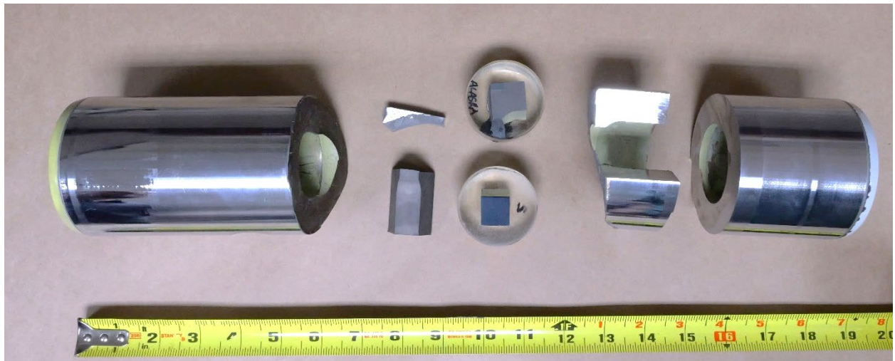
Figure 33. View of all the remnants and sections of the aft trunnion pin, taken after receipt and sectioning of the aft remnant (courtesy: Boeing EQA).
