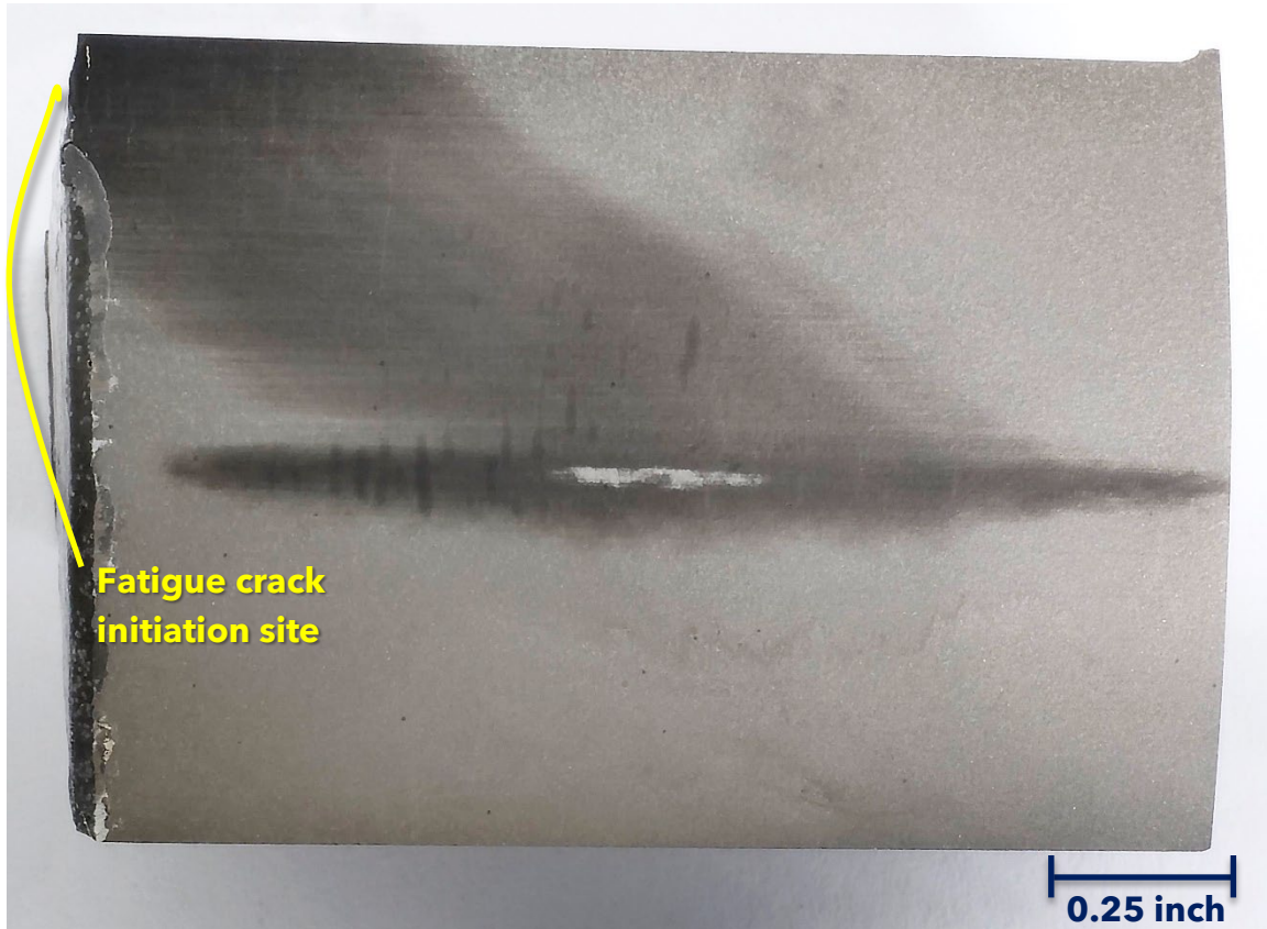
Figure 37. Images of the aft remnant of the aft trunnion pin showing temper etch surface contrast (courtesy: Boeing). The fracture surface is identified in the upper left.
