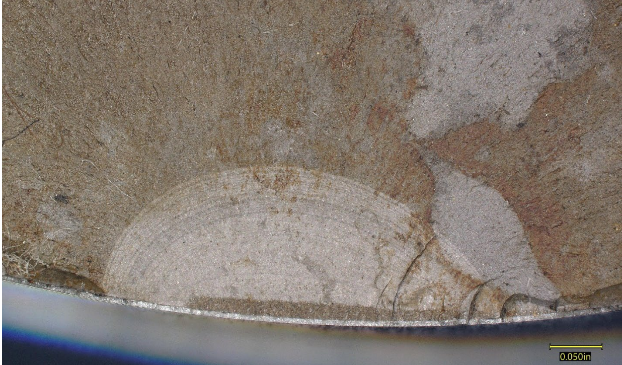
Figure 20. Close-up view of the thumbnail crack on the forward pin remnant.
