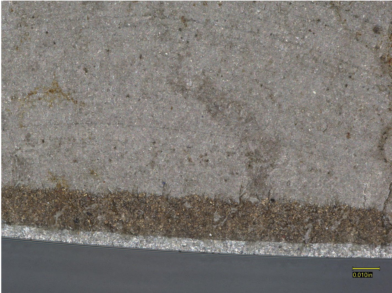
Figure 22. Closer view of the initiation region of the thumbnail crack, showing the Cr-plating surface layer and the darker subsurface intergranular layer.
