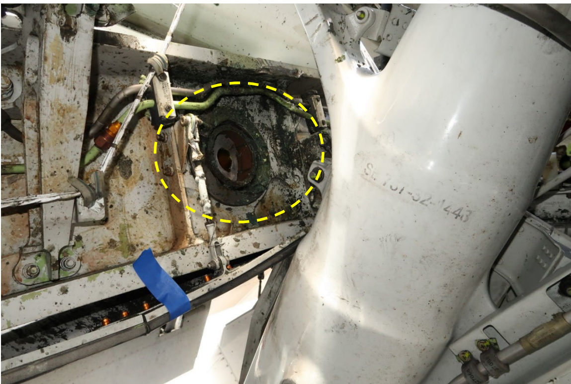
Figure 2. View of the fractured trunnion pin of the main landing gear on-scene.
