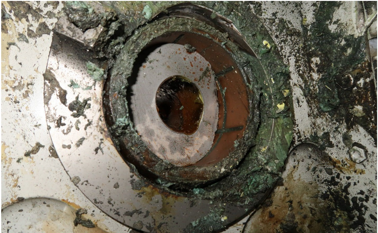
Figure 3. View of the fracture surface of the aft remnant of the aft trunnion pin remnant, on-scene.
