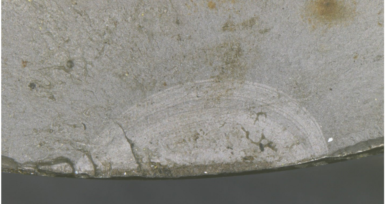
Figure 14. Closer view of the thumbnail crack in Figure 13 , showing crack arrest marks (courtesy: Boeing).
