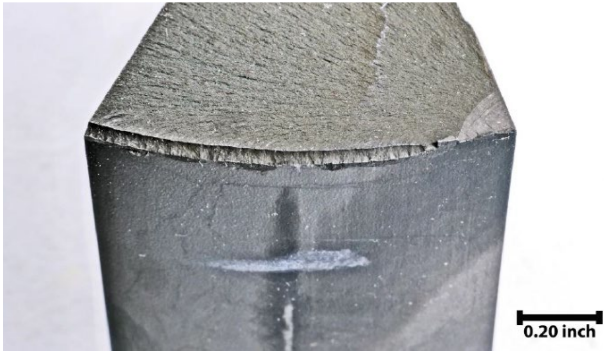
Figure 39. View of the temper etch indications relative to the sectioned thumbnail crack of the aft pin remnant (courtesy: Boeing).
