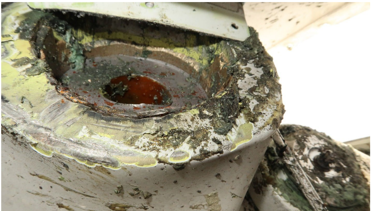
Figure 4. View of the mating fracture surface of the forward half of the aft trunnion pin, on-scene.
