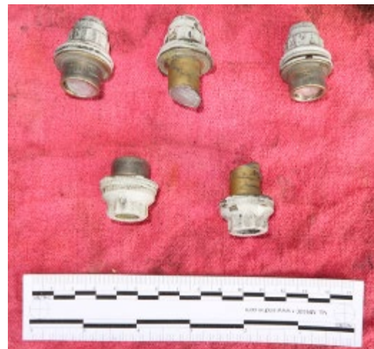
Figure 10. Sheared bolt fragments located within the wing main landing gear wing and wheel well area.
