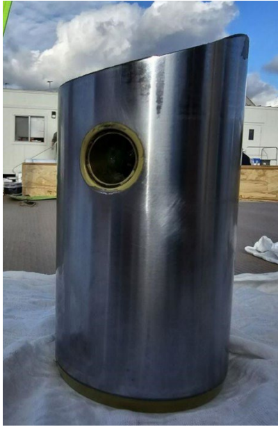
Figure 13. Side view of the trunnion pin half after removal from the outer cylinder. (Source: Troy Levanen, Alaska Airlines)
