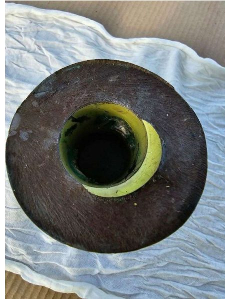
Figure 14. View of the fracture face of the trunnion pin half. (Source: Troy Levanen, Alaska Airlines)
