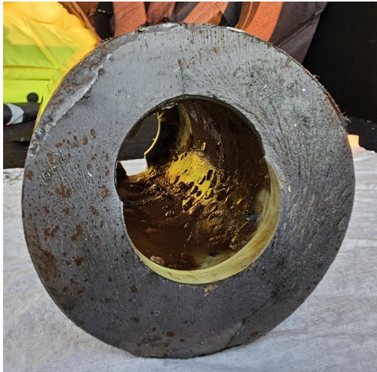
Figure 7. View of the trunnion pin fracture face. (Source: Alaska Airlines)
