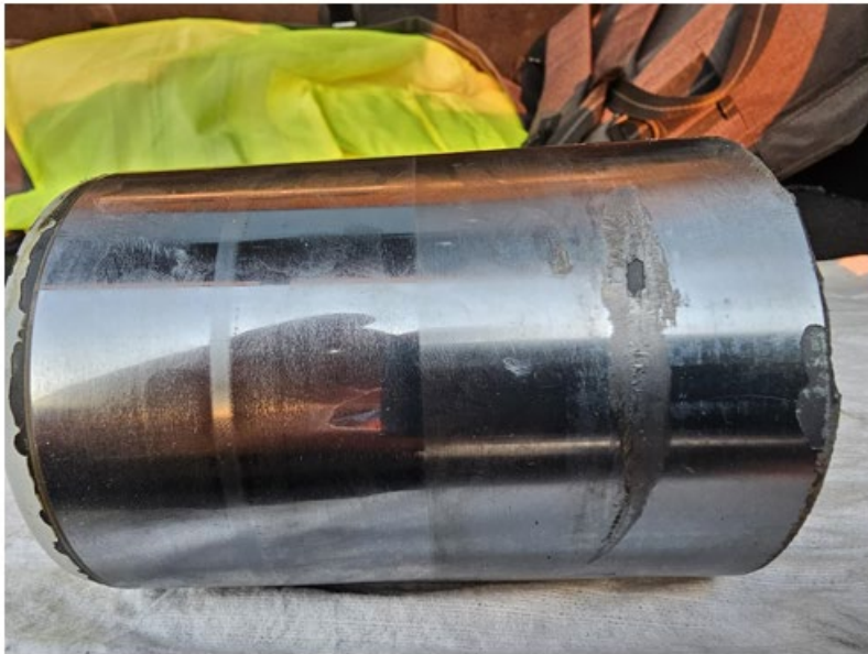
Figure 6. Two views of the trunnion pin half that was removed from the landing gear beam. (Source: Alaska Airlines,)
