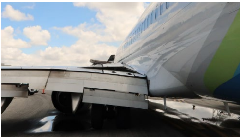
Figure 3. Aft view of the left wing showing upper wing panels displaced upward.
