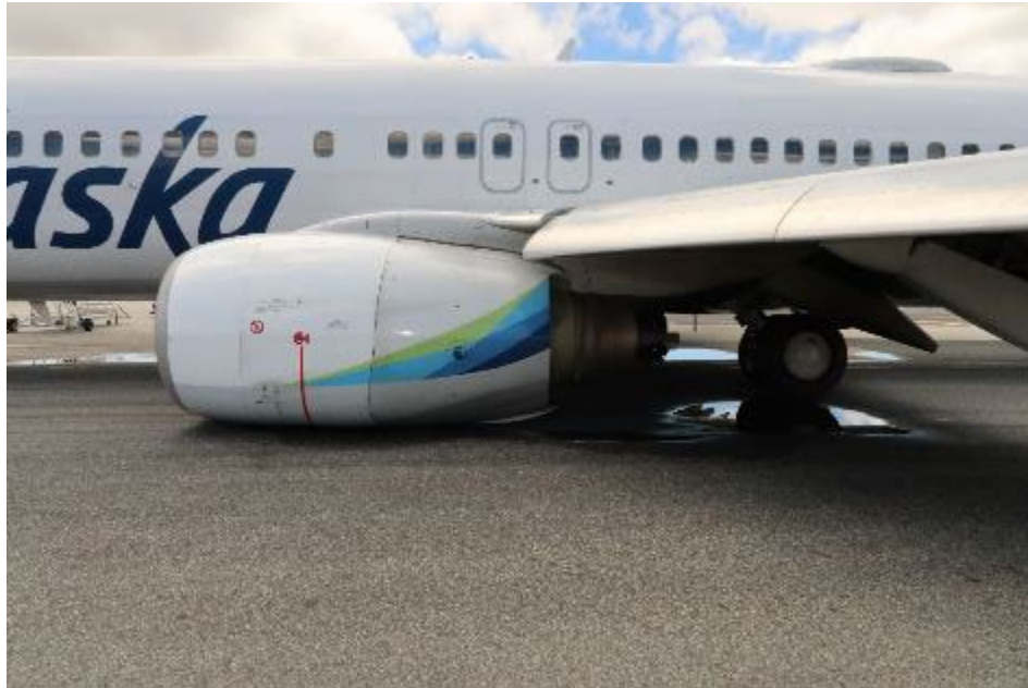
Figure 1. Left side view of the airplane resting on the left engine nacelle and left main landing gear displaced aft.
