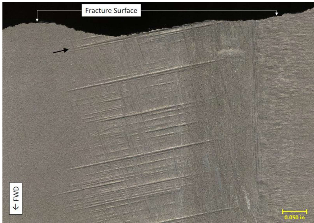
Figure 8 - A digital microscope image of the lower surface of the forward lower lock link piece adjacent to the fracture origin area. Visible horizontal and vertical scratches were observed. The fracture plane was oriented parallel to a horizontal scratch as indicated by the black arrow. 28
