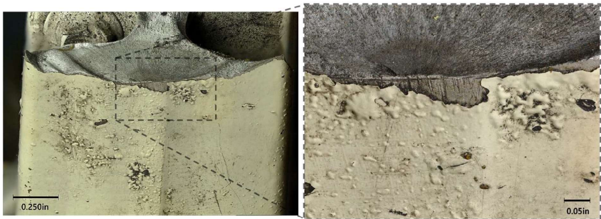
Figure 6 – Digital microscope images of the fracture origin area and adjacent lower surface on the forward piece. 25
