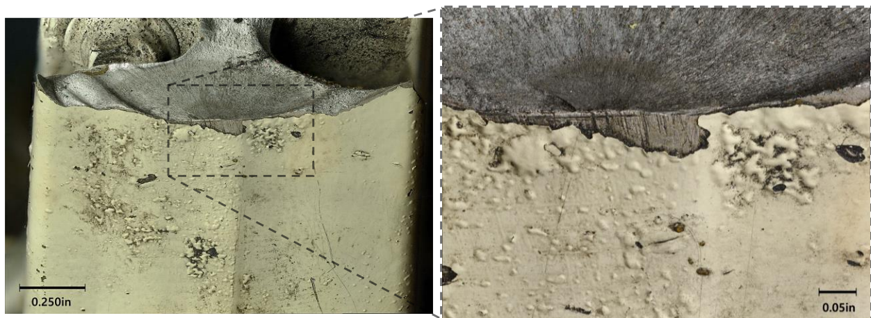
Figure 4. Digital microscope images of the fracture origin area and adjacent lower surface on the forward piece, as received. Horizontal and vertical scratch features were observed near the origin on the adjacent surface beneath the paint layer.
