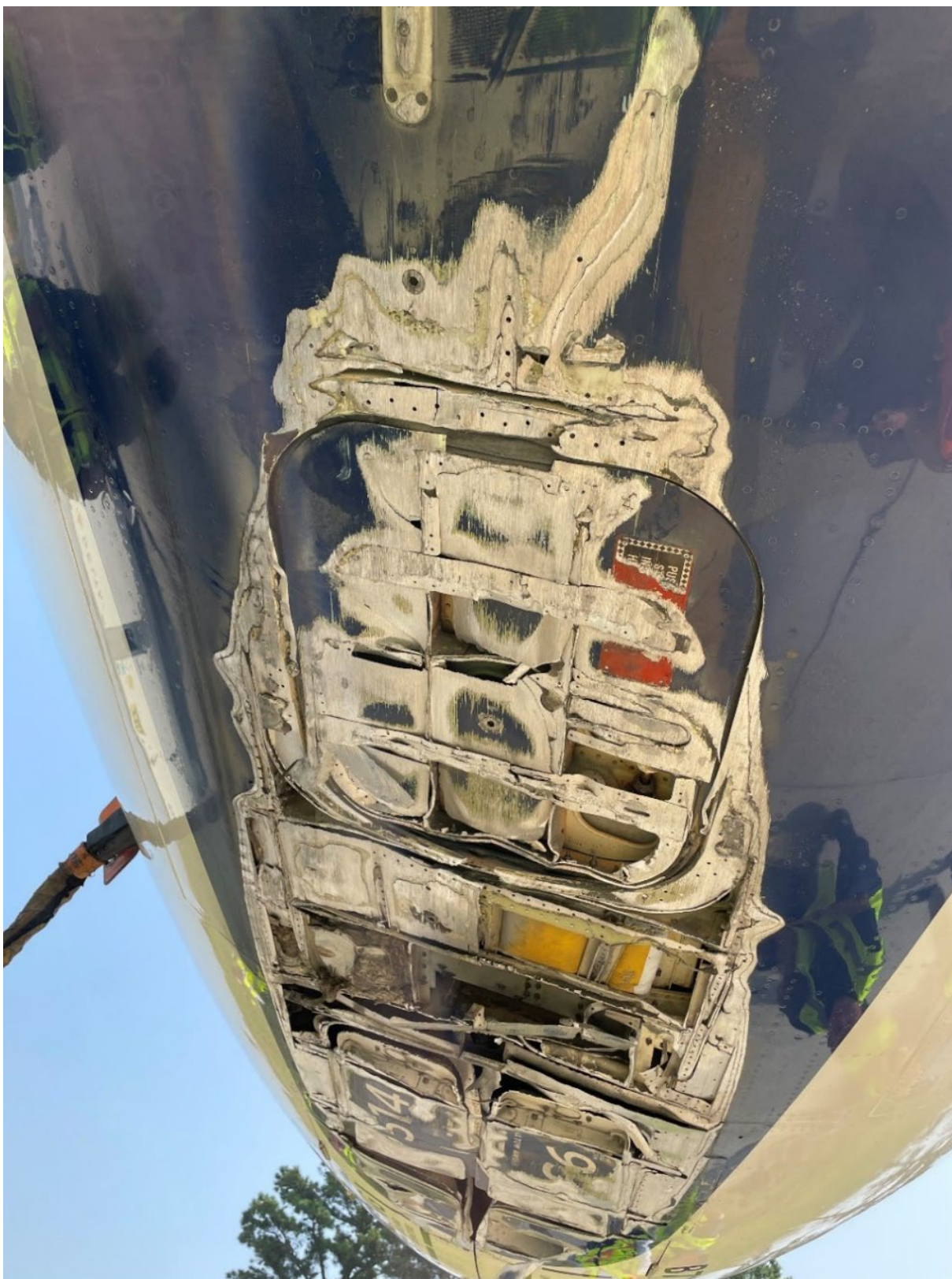
Figure 6: Abrasion damage to the lower fuselage skin, frames, and doors (view is looking forward towards nose).
