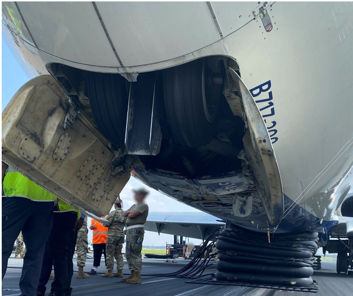
Figure 9: Nose gear wheel position during aircraft recovery from the runway. (Photograph used with permission from the FAA)
