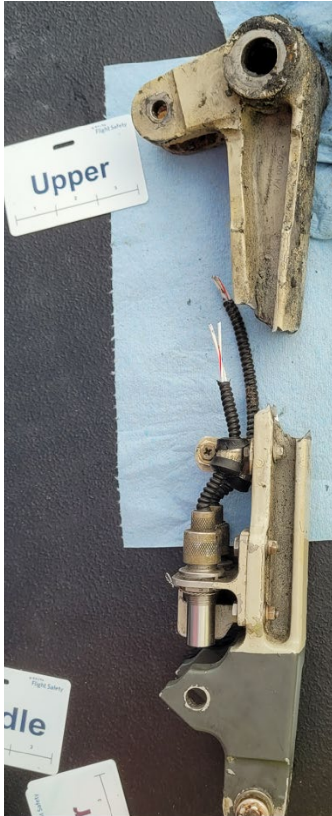
Figure 7: Fractured upper lock link.
