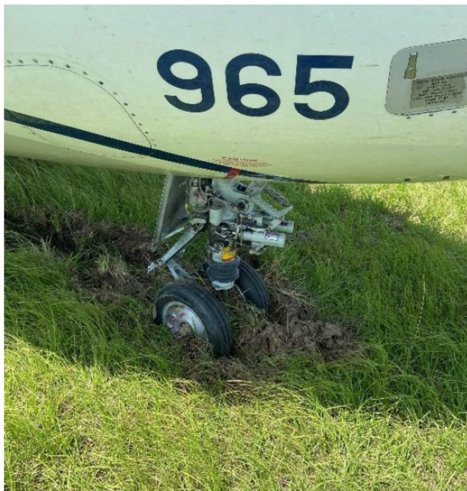
Photograph 5 - View of Nose Landing Gear (Courtesy MHIRJ)
