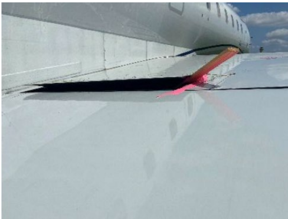
Photograph 4 - View of Damage to Flap Skin (Courtesy MHIRJ)
