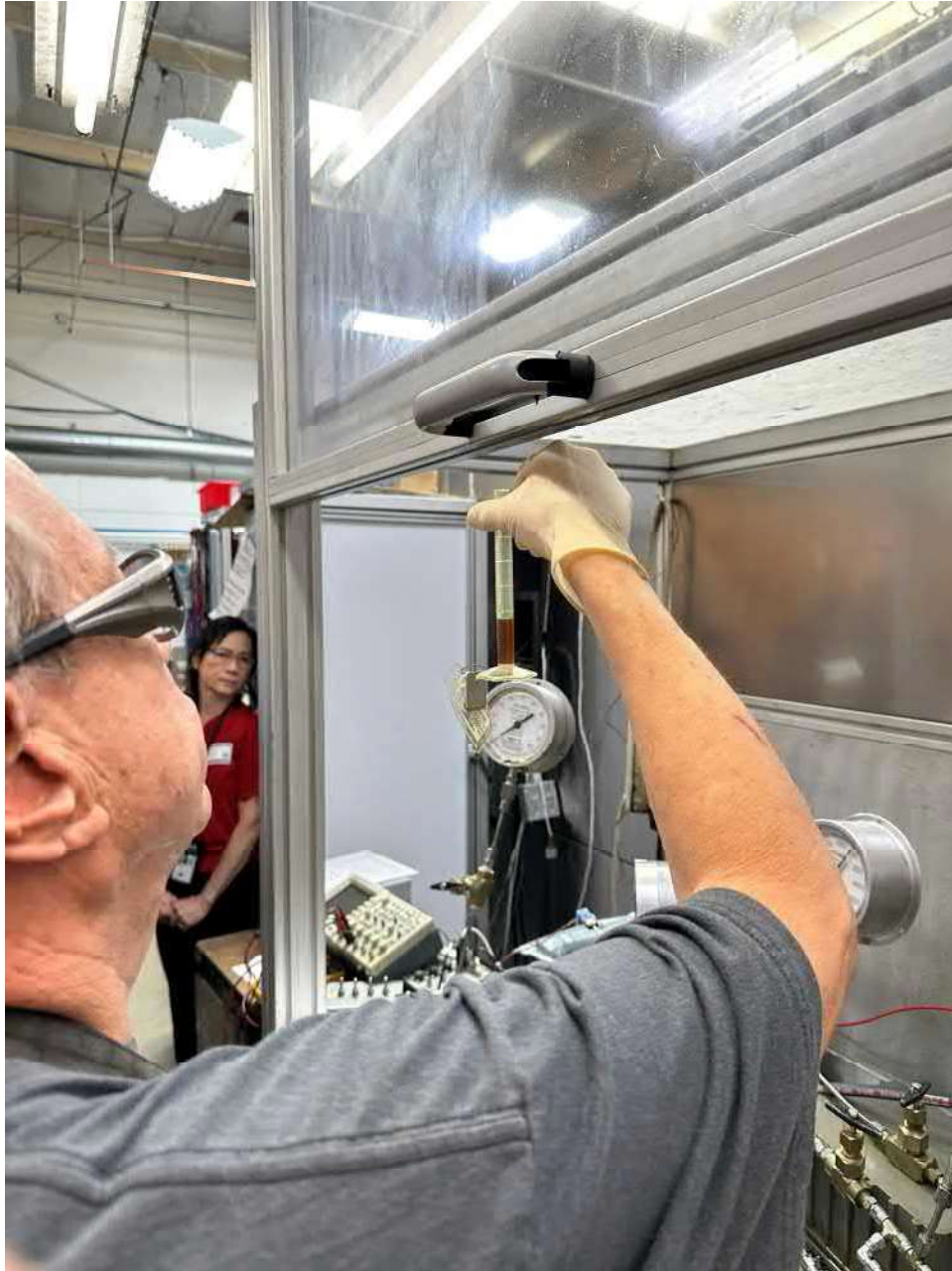
View of technician making visual assessment of volumetric value of internal leakage.
