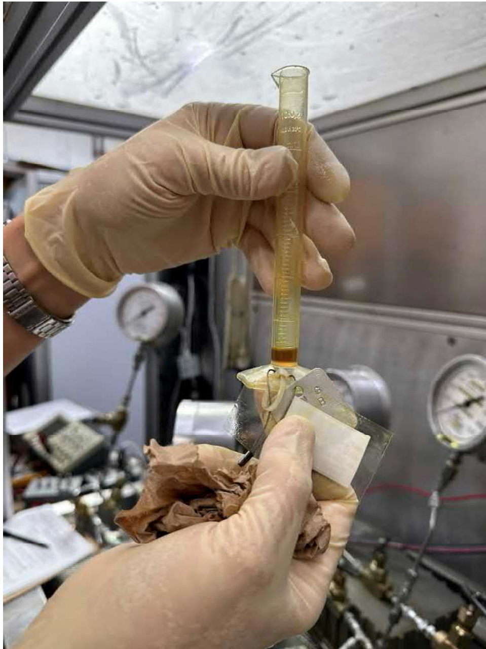
View of a volumetric beaker used to assess the amount of internal leakage during the performance of the ATP.
