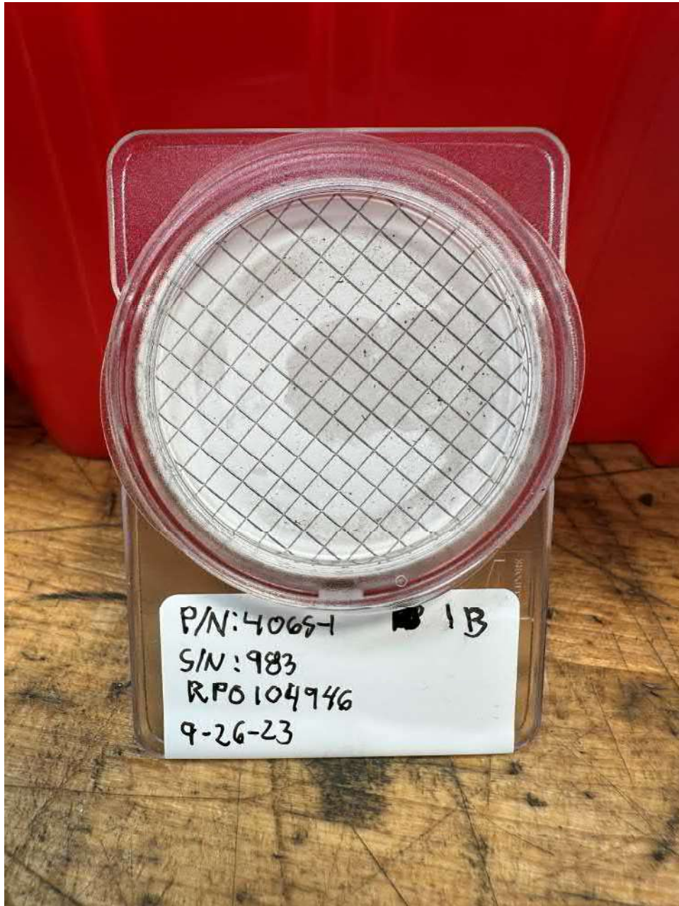
View of the inbound filter patch showing evidence of particulate FOD (deemed irrelevant in this case) from the aircraft hydraulic system upon which the component was installed.
