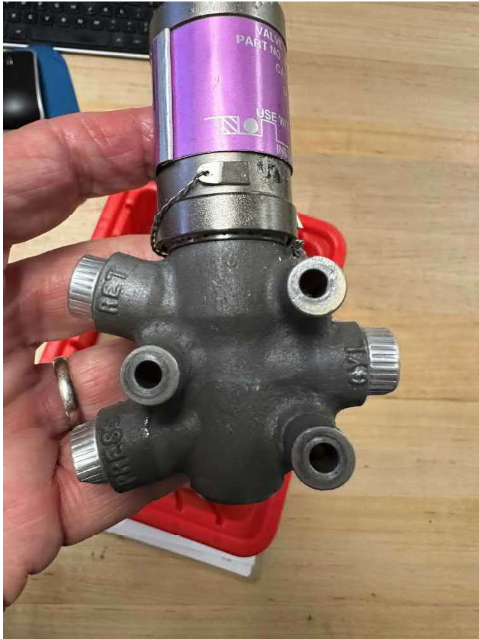
View of mounting holes from the other side.
