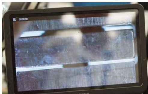
Armature Gaps under 10x Magnification – No FOD
