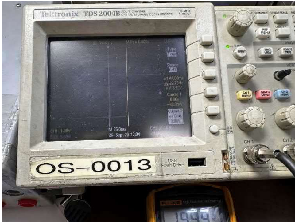
View of oscilloscope screen during performance of the timing tests for actuation/deactuation.
