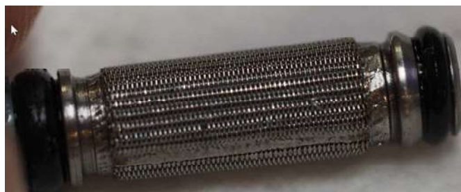
Inlet Filter – No FOD or Debris Observed
