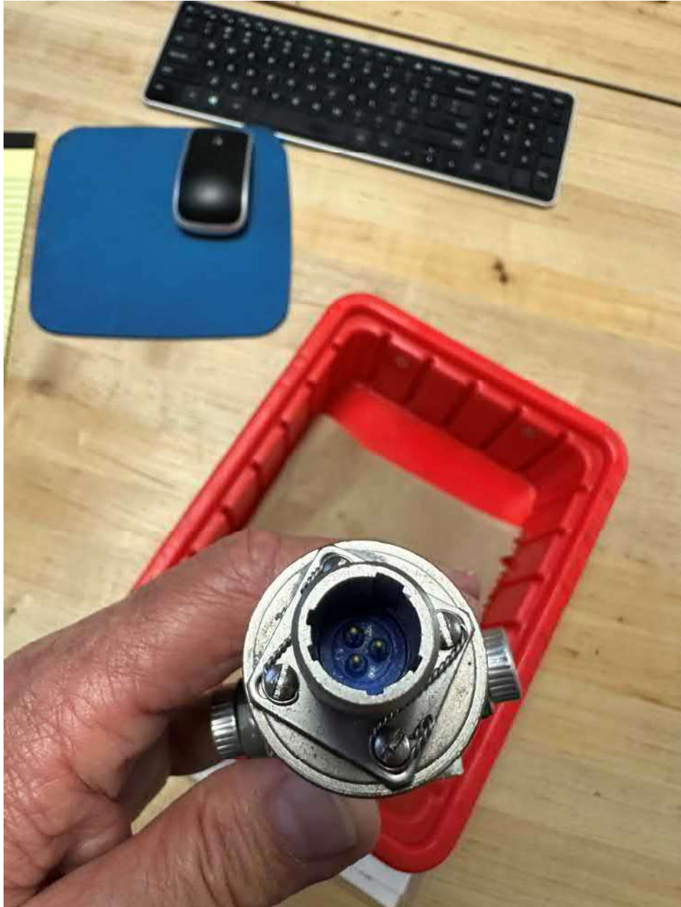
View of connector on solenoid showing pins and rubber insulator.
