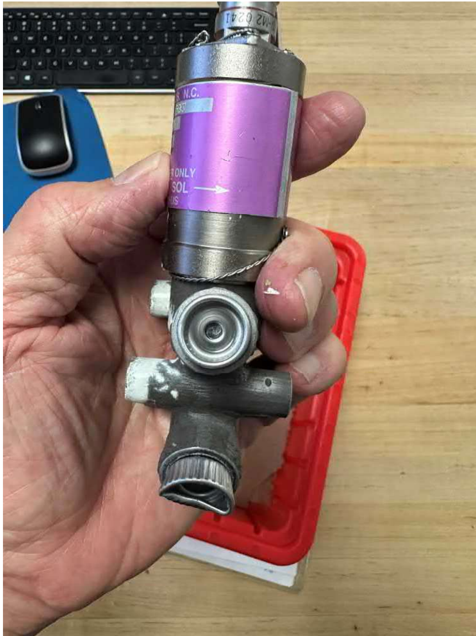
View of the capped return port.
