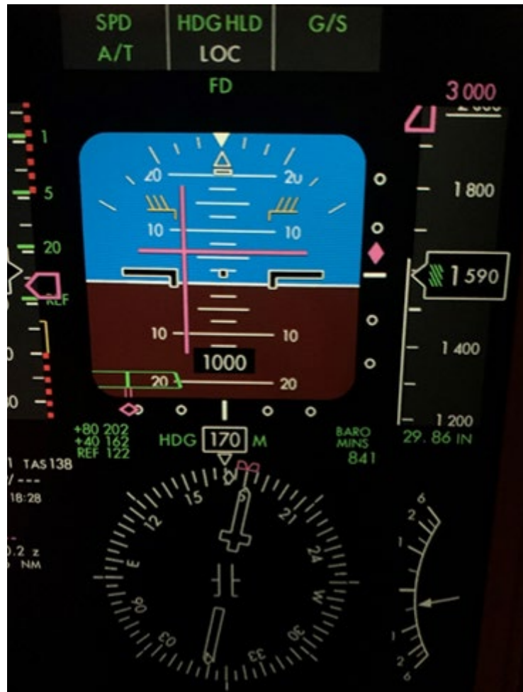
Figure 10. Simulator PFD as viewed approaching runway 18R.
