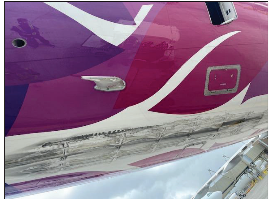
Figure 1 – Tail Strike Damage between FR61-69 and S-39L to S-42R Actual Pictures (Sheet 3 of 6)
