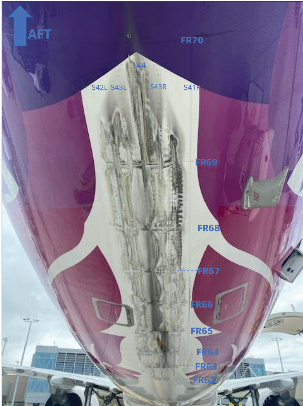
Figure 1 – Tail Strike Damage between FR61-69 and S-39L to S-42R Actual Pictures (Sheet 1 of 6)
