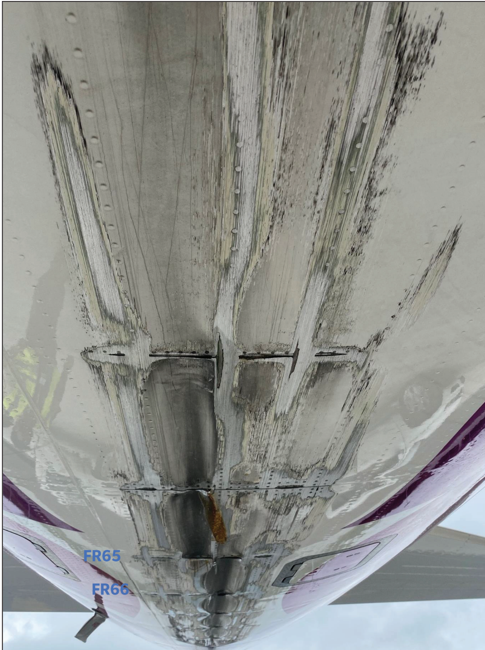
Figure 1 – Tail Strike Damage between FR61-69 and S-39L to S-42R Actual Pictures (Sheet 3 of 6)
