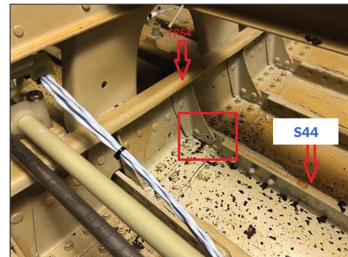
Figure 1 – Tail Strike Damage between FR61-69 and S-39L to S-42R Actual Pictures (Sheet 5 of 6)
