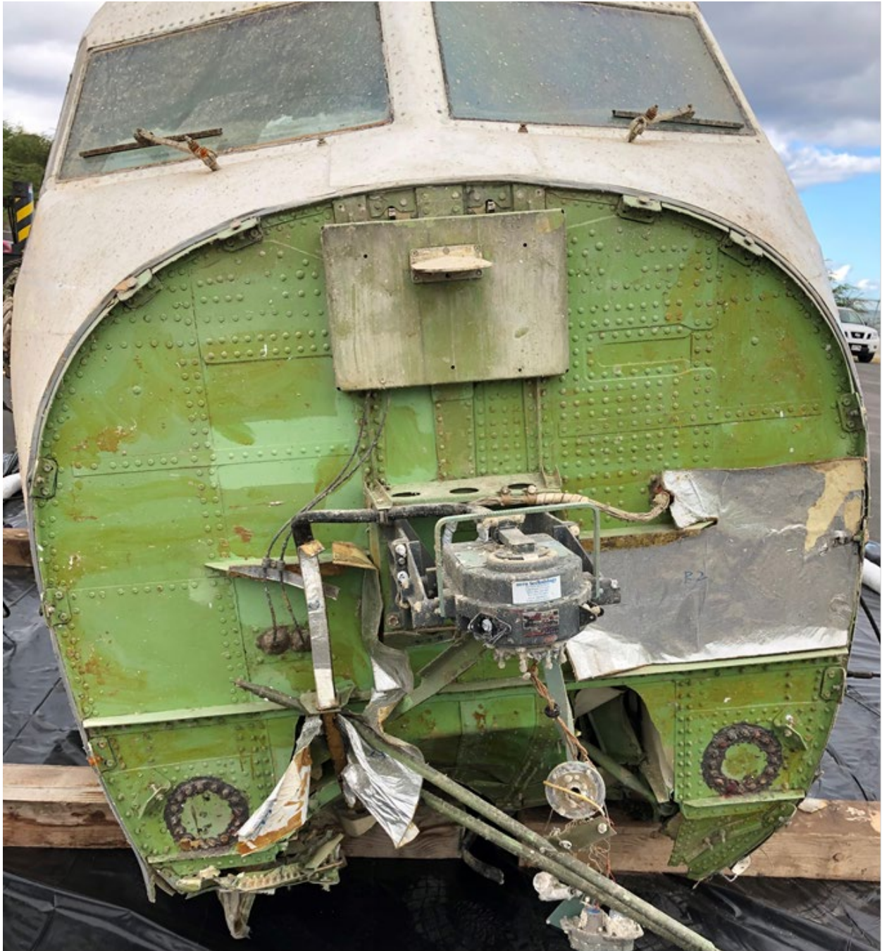
Figure 18. Forward Bulkhead/Radar Mounting
