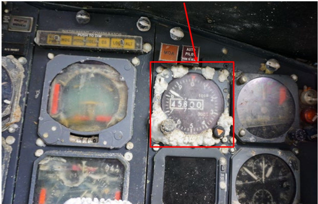
Figure 5. First Officer's Altimeter Noted by Arrow and Box
