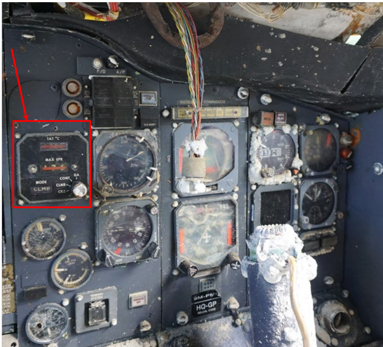
Figure 4. First Officer's Instrument Panel with Thrust Panel Noted by Arrow and Box
