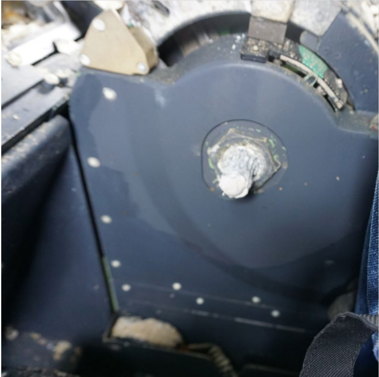
Figure 14. Left Stabilizer Wheel Attach Point/Stab Trim Position Indicator
