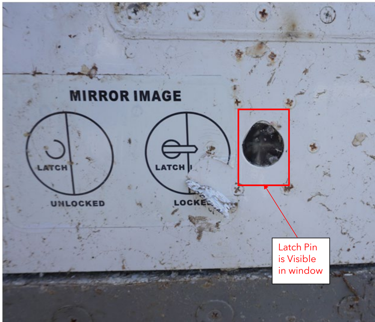
Figure 16. Upper Cargo Door Latch Pin
