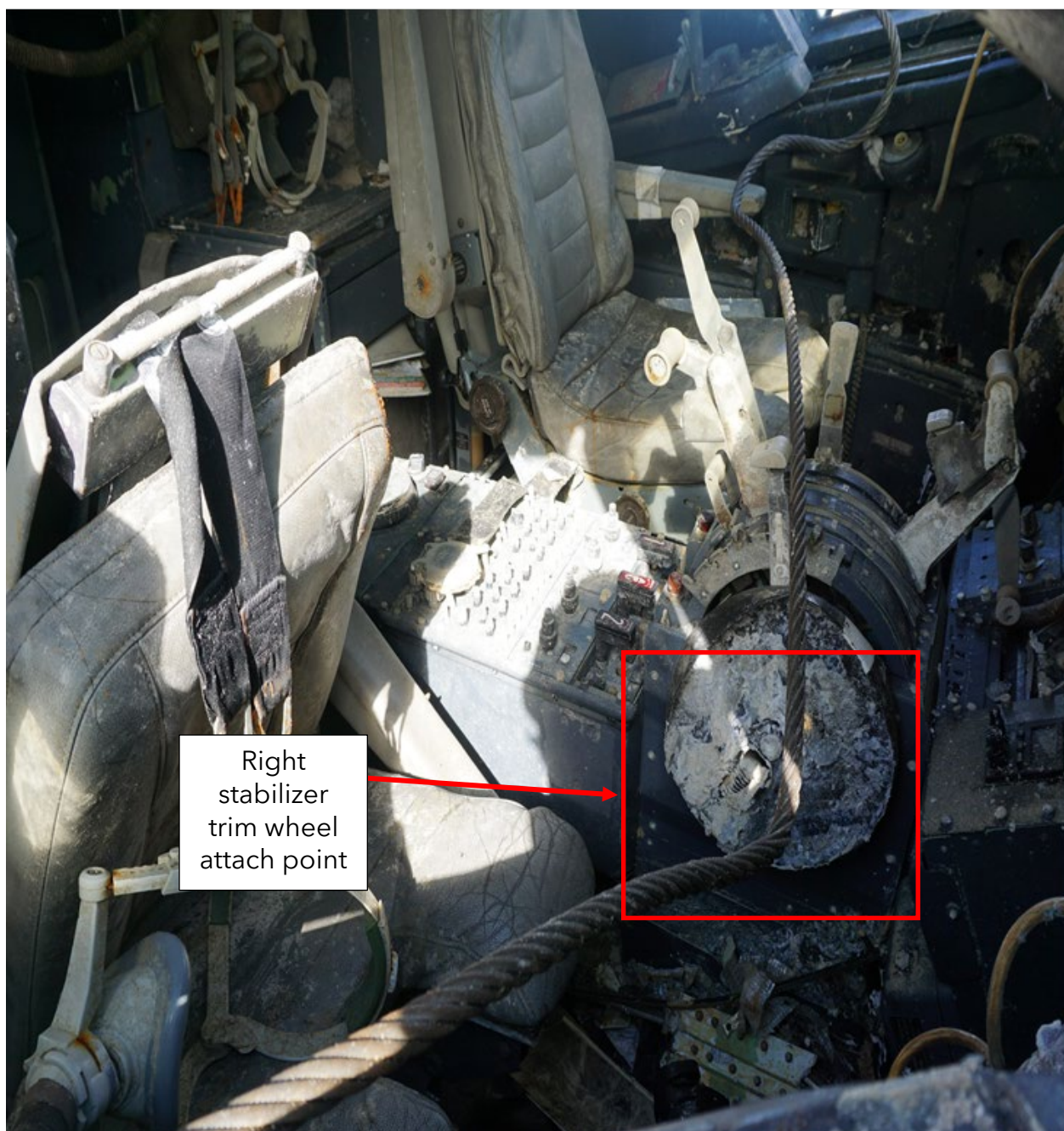
Figure 13. Right Stabilizer Trim Wheel Attach Point Location
