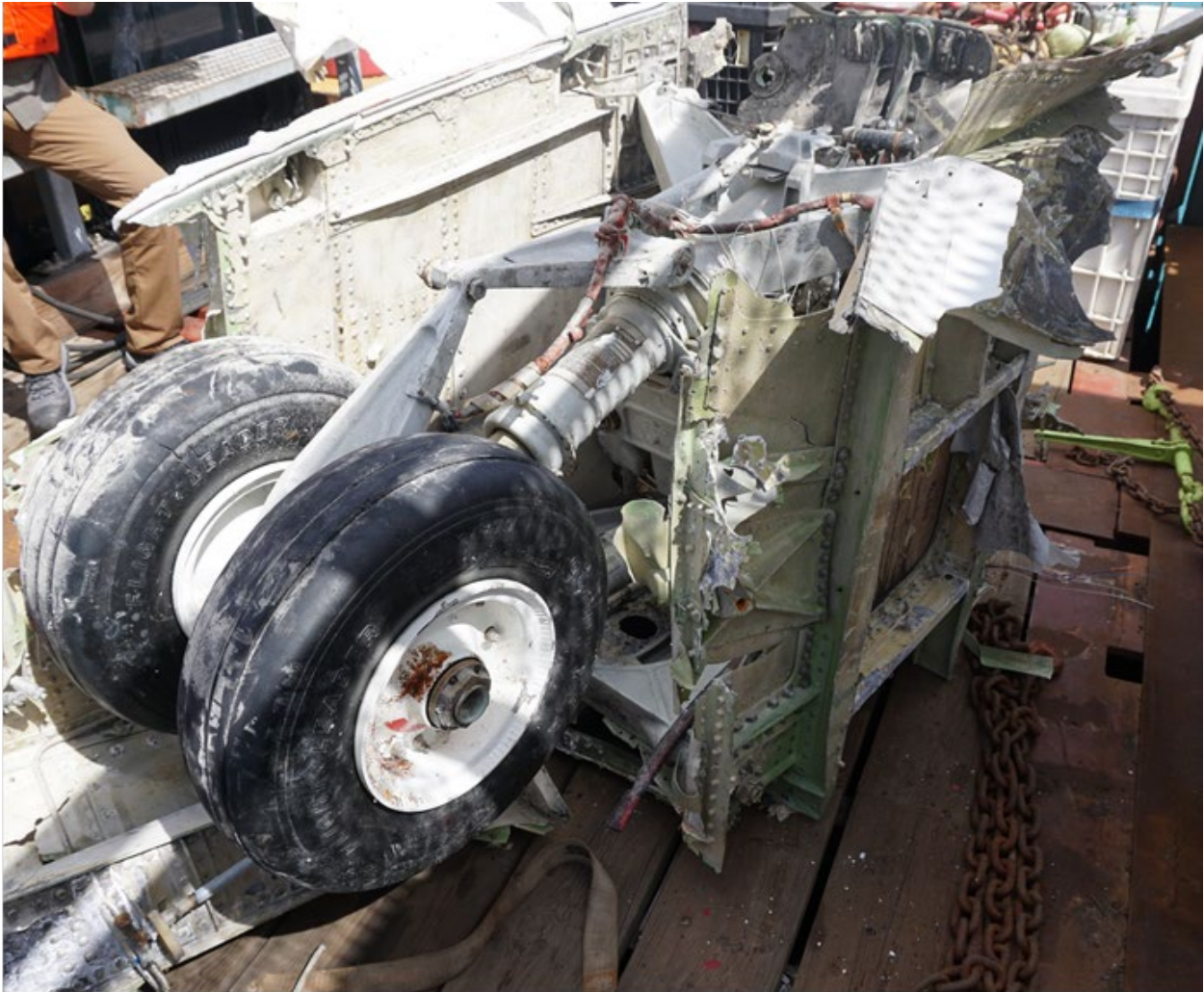
Figure 17. Nose Gear and Attach Box Structure
