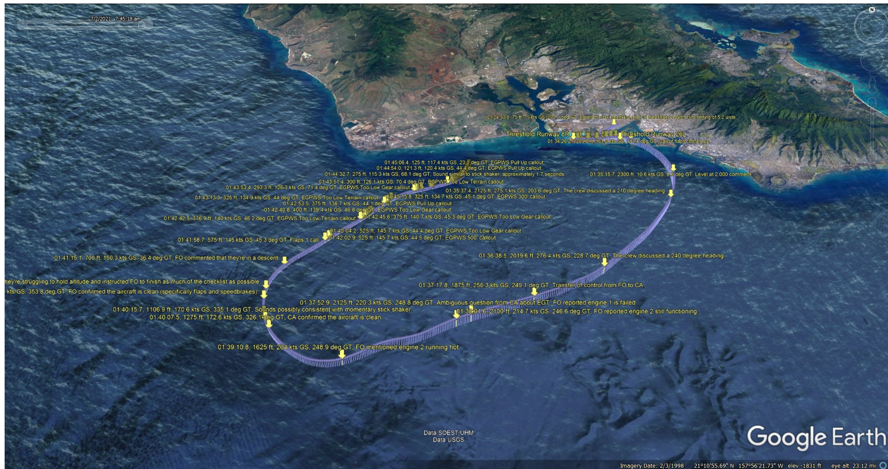
Figure 4: Addition of paraphrased CVR events to FAA ADS-B data depicting N810TA accident flight sequence from ground taxi to runway 8R through the takeoff, initial climb, and multiple altitude hold, course change, and descent segments to the ocean surface. Aircraft direction of travel during the approximately 12-minute flight is in the clockwise direction. Due north is toward the top of the page. Parametric data indicate time (HST hh:mm:ss), altitude, groundspeed, and ground track heading.
