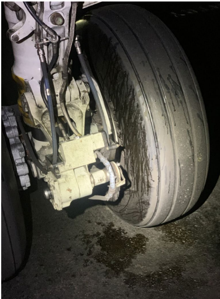
Photo 1: Fluid on left main landing gear tire and surrounding ground. 13
