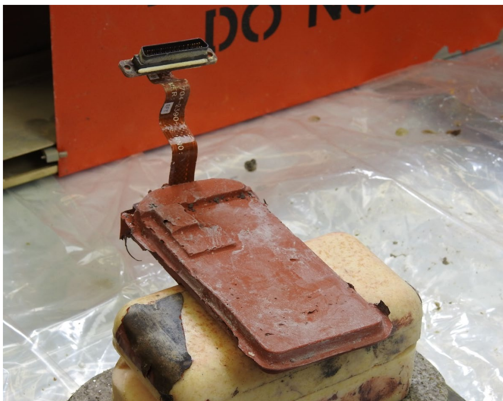
Figure 2. Memory module removed from the recorder.
