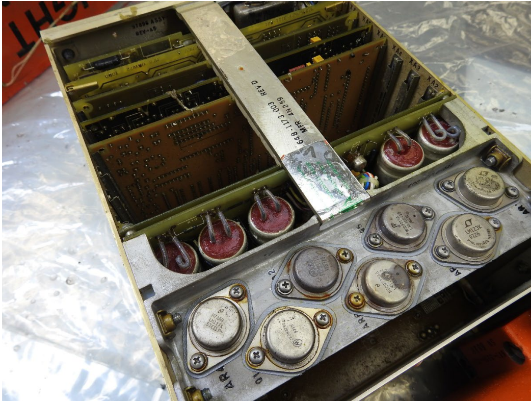
Figure 6. Processor and data acquisition cards inside FDR.
