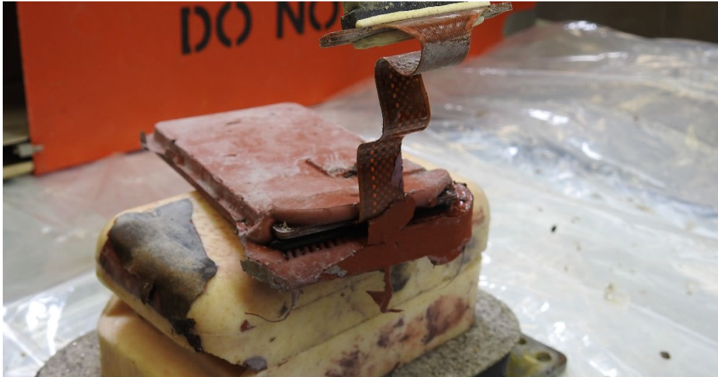
Figure 3. Memory module showing defective RTV sealant around the connector end of the board.
