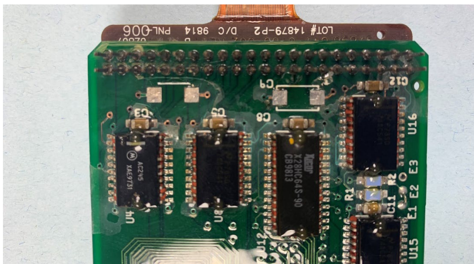
Figure 5. Detail view of area where two damaged capacitors were removed prior to readout.
