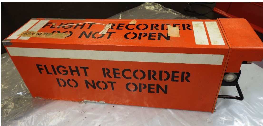
Figure 1. Exterior of flight data recorder after removal from water.
