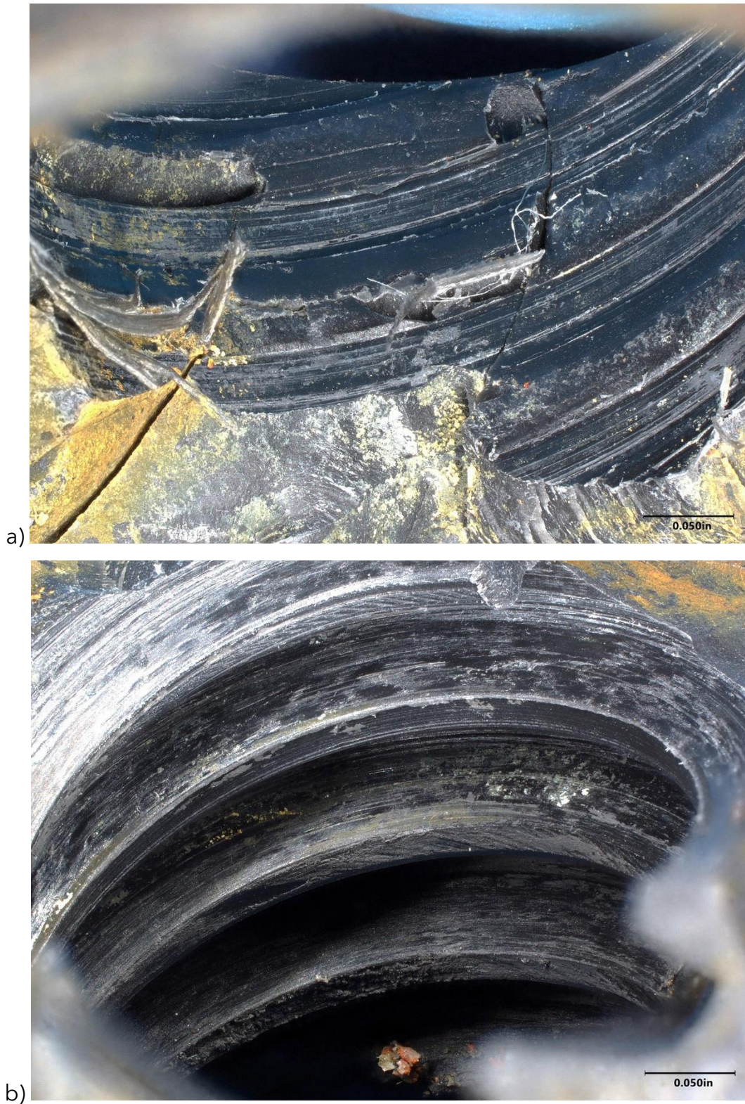
Figure 8. Images of the jack nut threads; a) stripped threads in the large-diameter portion with the locking slots and b) intact threads on the smooth-barrel small-diameter portion.
