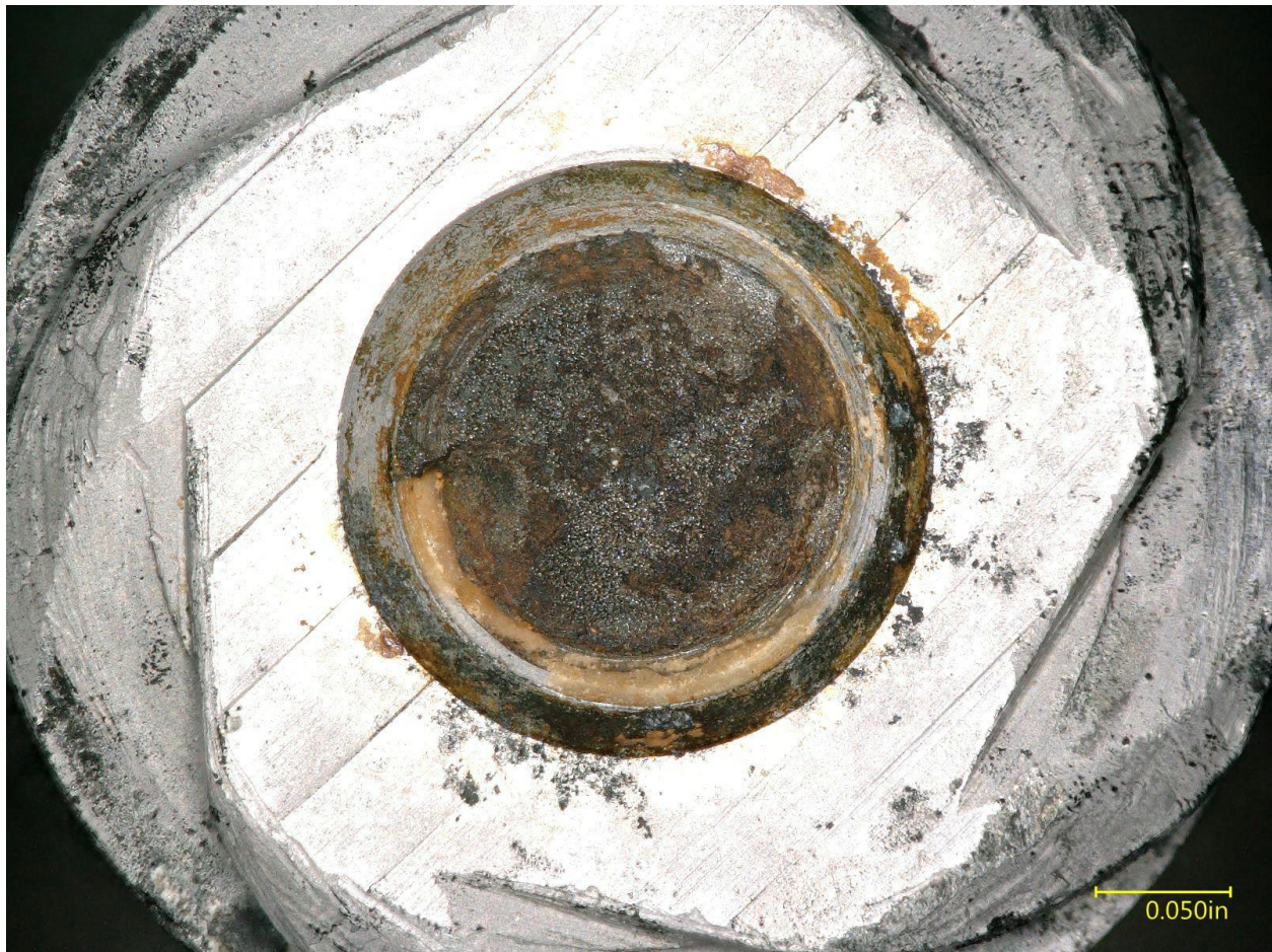
Figure 9. Image of the fractured attachment screw used to secure the stop washer to the end of the jack screw. The fracture had a rough appearance and a conical profile, consistent with an overstress fracture.
