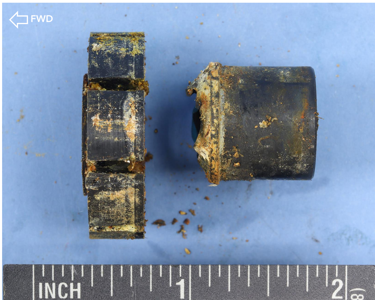
Figure 5. Image of the fractured nut after disassembly.
