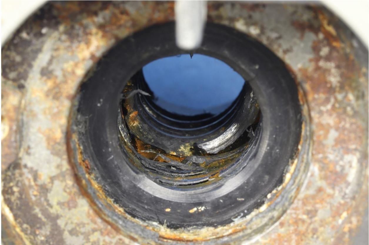
Figure 3. Image of the nut prior to disassembly. The nut was fractured in the transverse plane.
