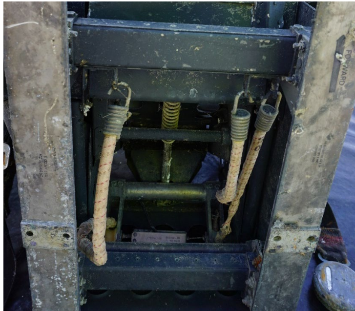
Figure 8 View of first officer seat from the bottom after removal from the airplane.
