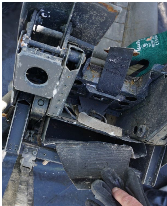
Figure 9 First officer seat as viewed from the front looking back, showing damage to stowage compartment.
