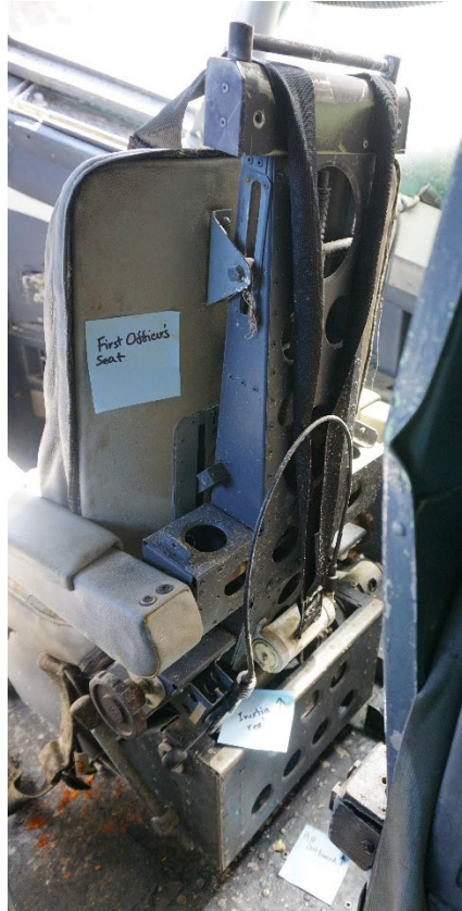
Figure 11 First officer inertia reel after removal of seatback cover.
