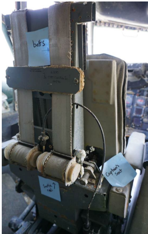
Figure 10 Captain inertia reels after removal of seatback cover.
