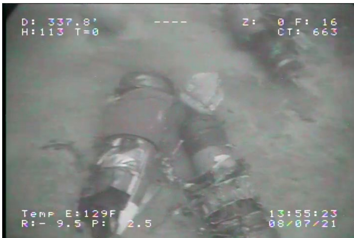
Figure 12. Engine cores and one thrust reverser
