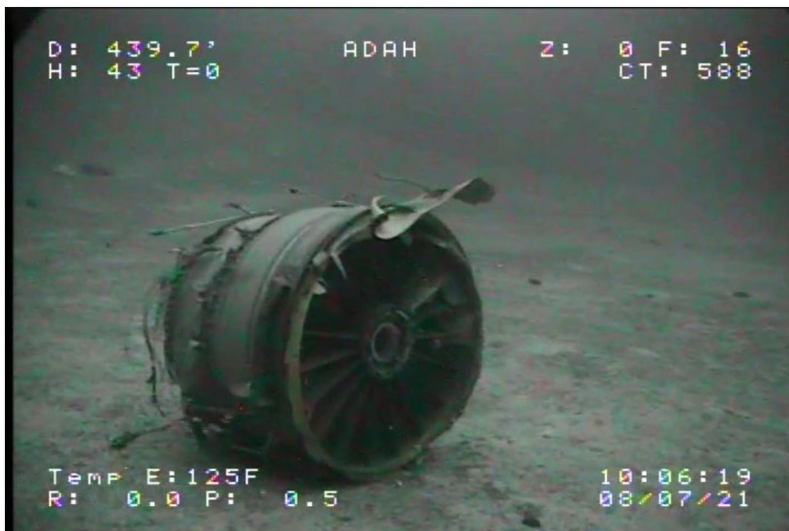
Figure 14. Engine #2 inlet case
