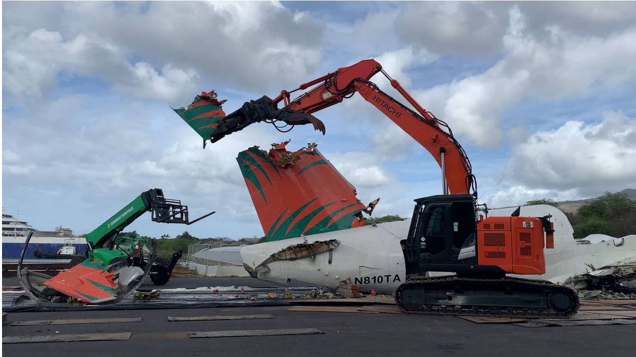
Figure 36. Vertical stabilizer being removed from the fuselage
