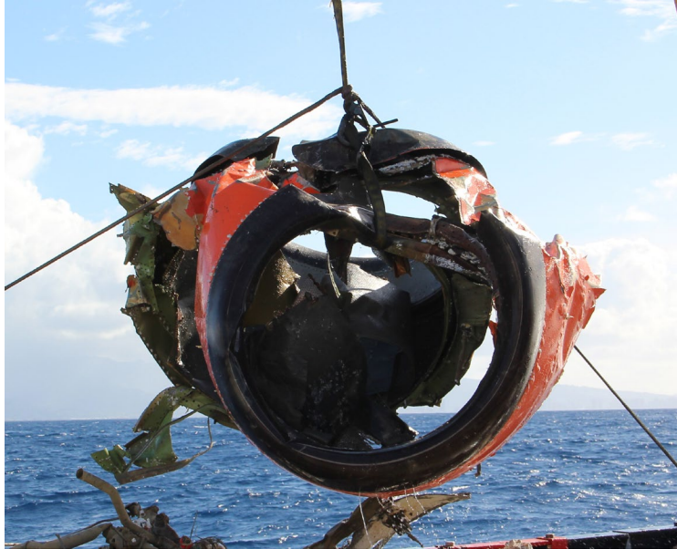
Figure 20. Recovered engine nose cowls
