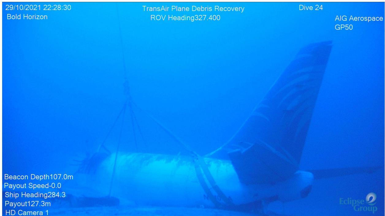
Figure 28. Aft fuselage rigging under tension
