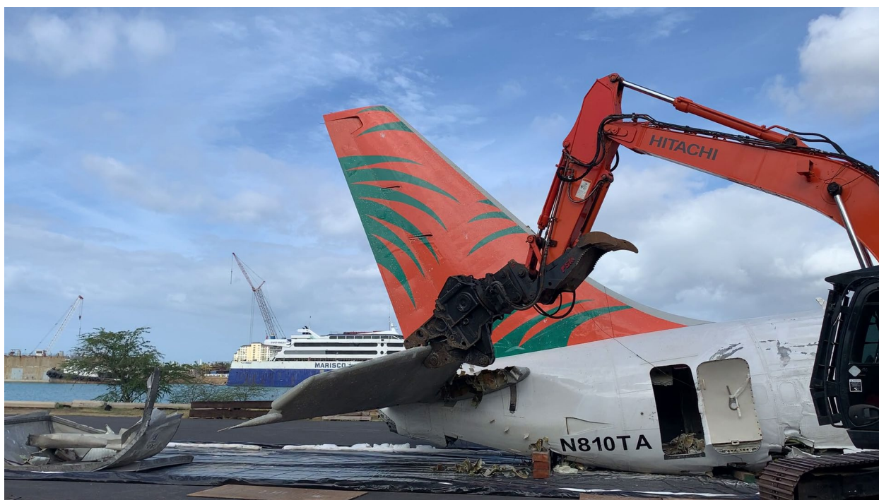
Figure 35. Right horizontal stabilizer being cut from the fuselage
