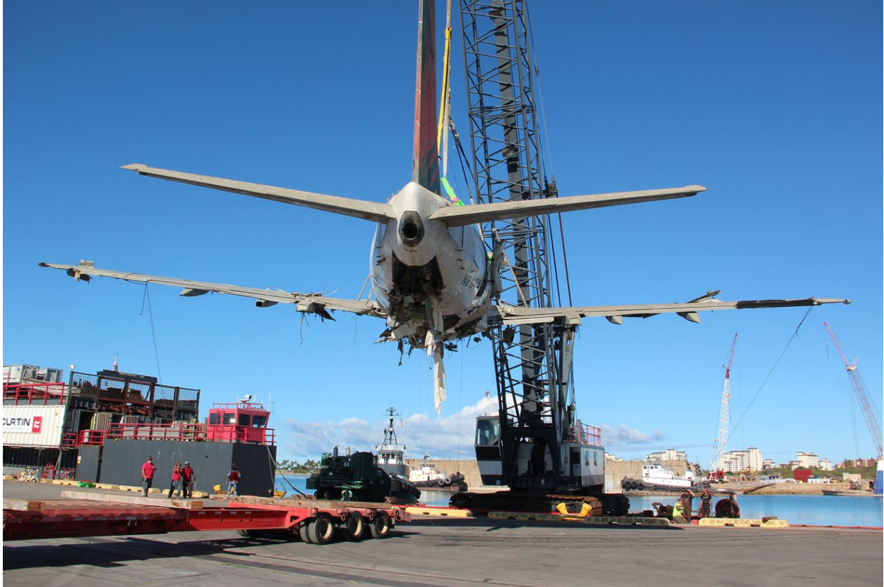
Figure 31. Aft fuselage transfer to pier
