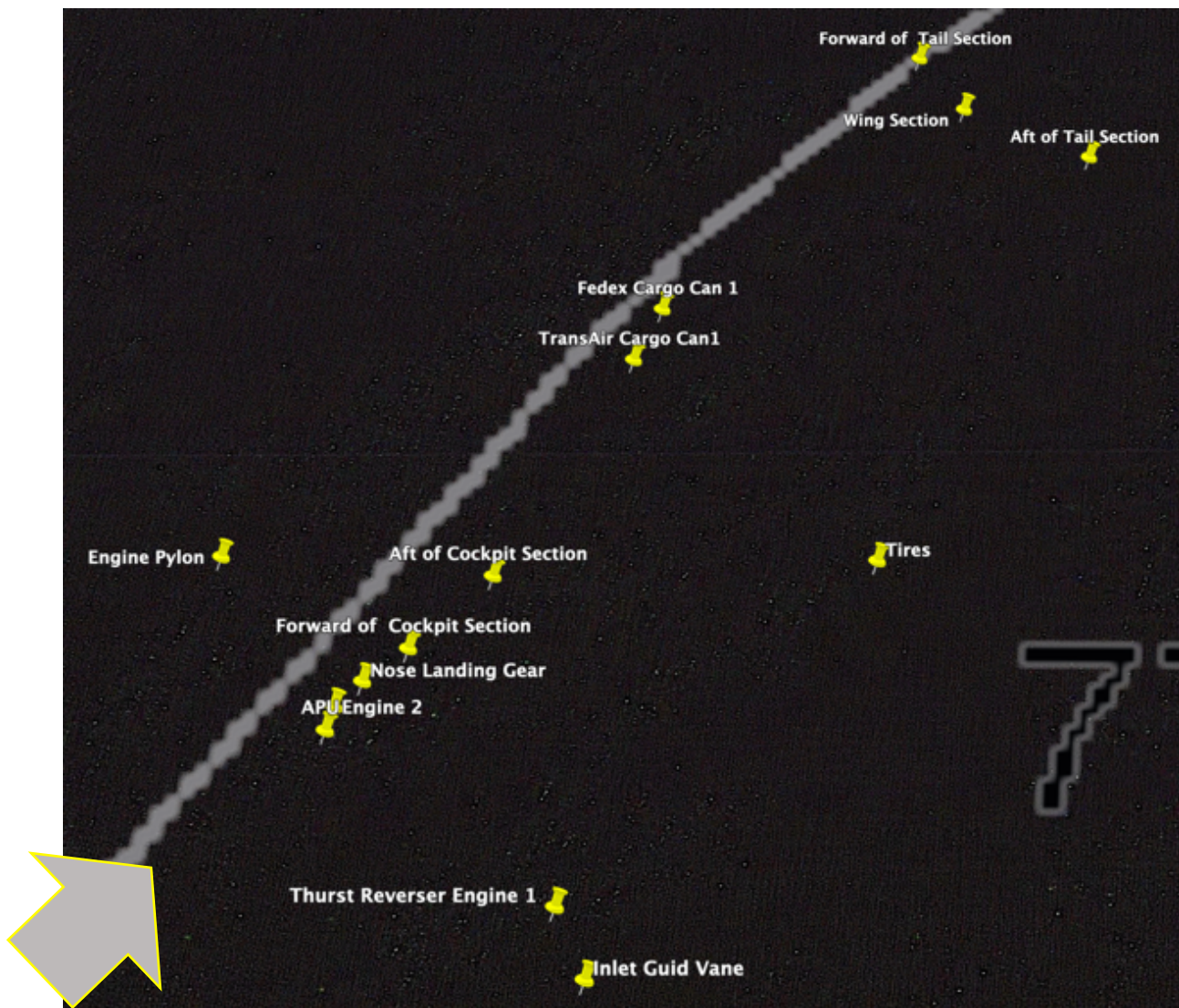
Figure 5. Relative locations of debris determined by survey ROV.
