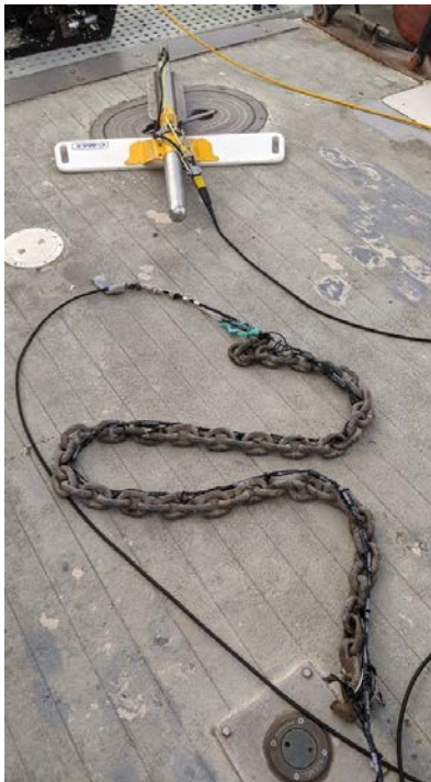
Figure 12 Chain Attached the Side Scan Sonar Tow Cable
