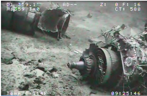
Figure 36. #2 Engine on right shows accessory gearbox
