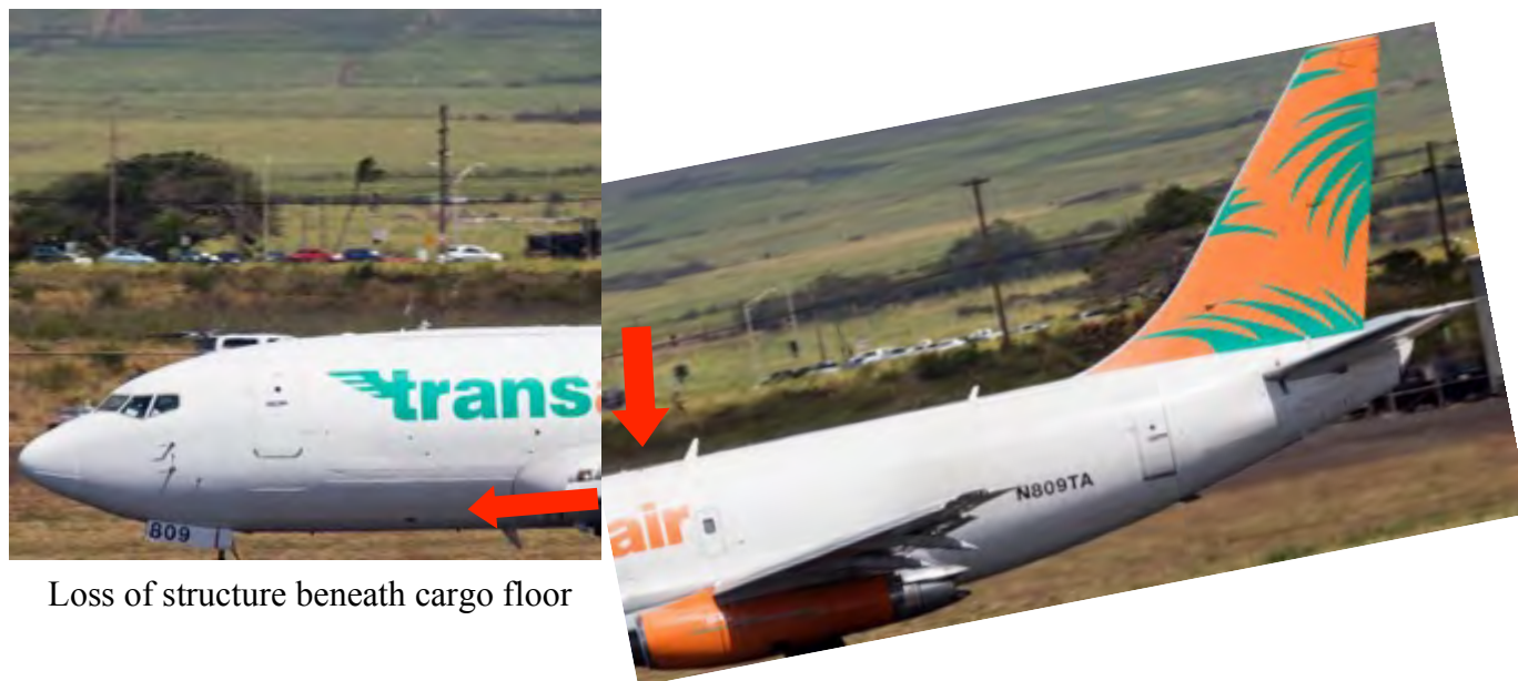
Figure 22. Relative damage in portions of fuselage
