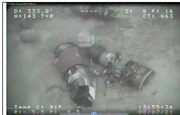
Figure 30. #1 T/R on left. #1 Engine on right
