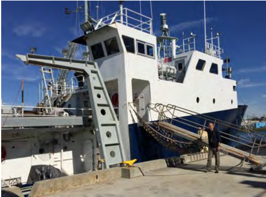
Figure 10. The BH Starboard J-Leg lifting point is shown above
