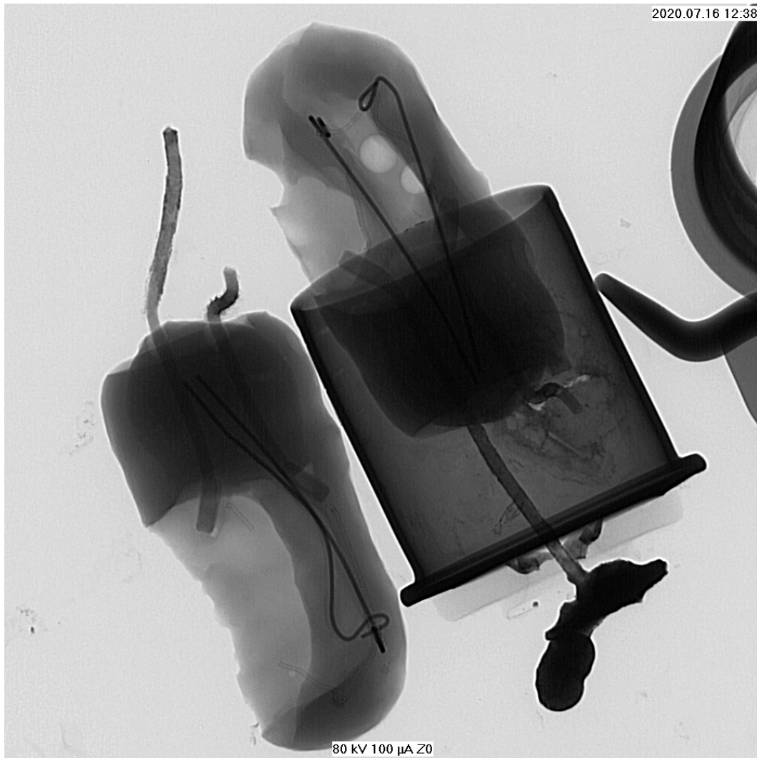
Figure 35. Radiograph of Column 8 Row 4 bulbs of Caution/Advisory Annunciator Panel.
