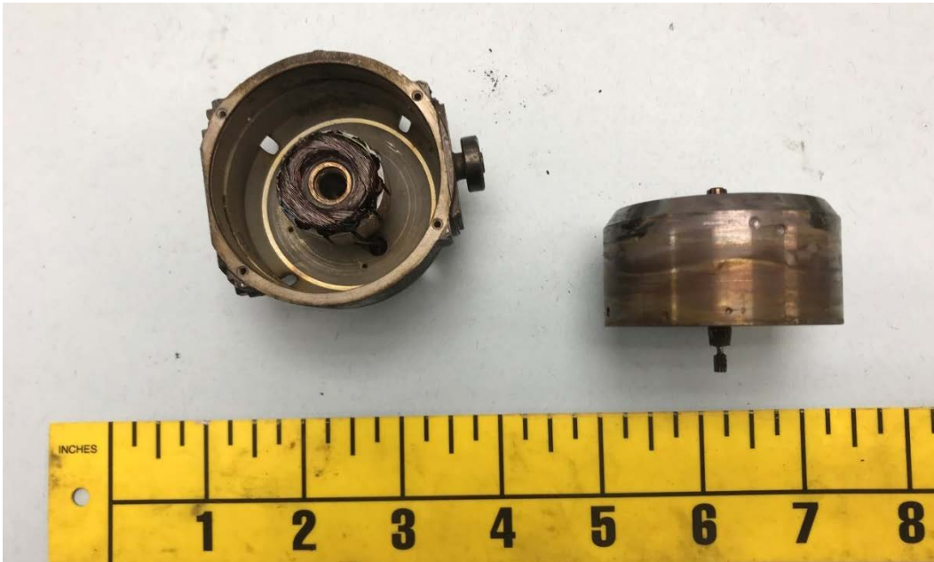
Figure 48. Gyro (mass and case) from Standby Attitude Indicator.
