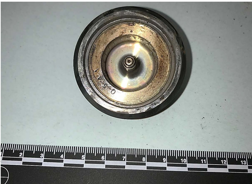
Figure 47. Top of gyro rotational mass from Standby Attitude Indicator
