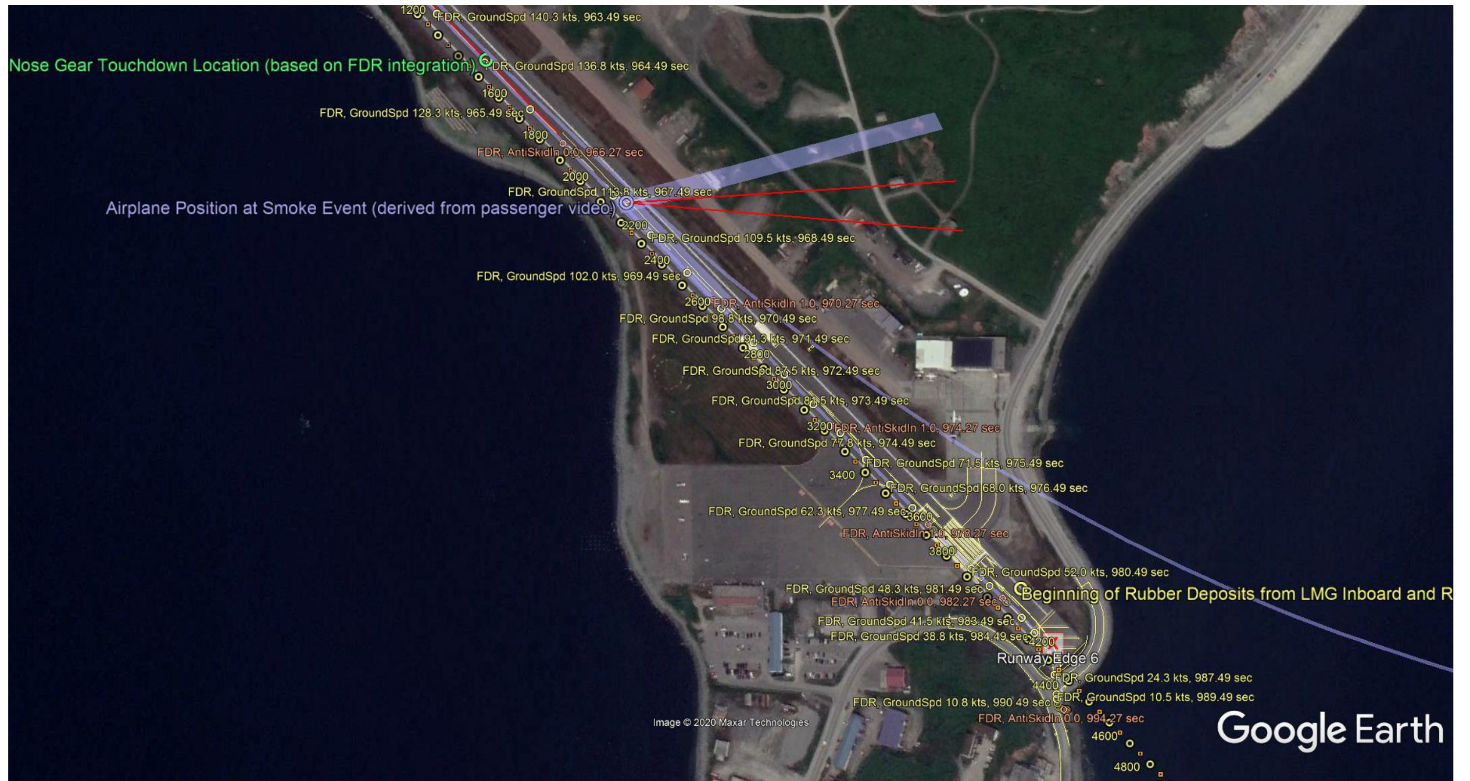
Figure A1.5: Planform view of runway 13 departure end with N686PA FDR ground speed in knots (yellow) and FDR anti-skid fault parameters (orange, 1=fault) annotated along the airplane ground track. True north is toward the top of the page. The FDR time values correspond to FDR SRN – 156000.
