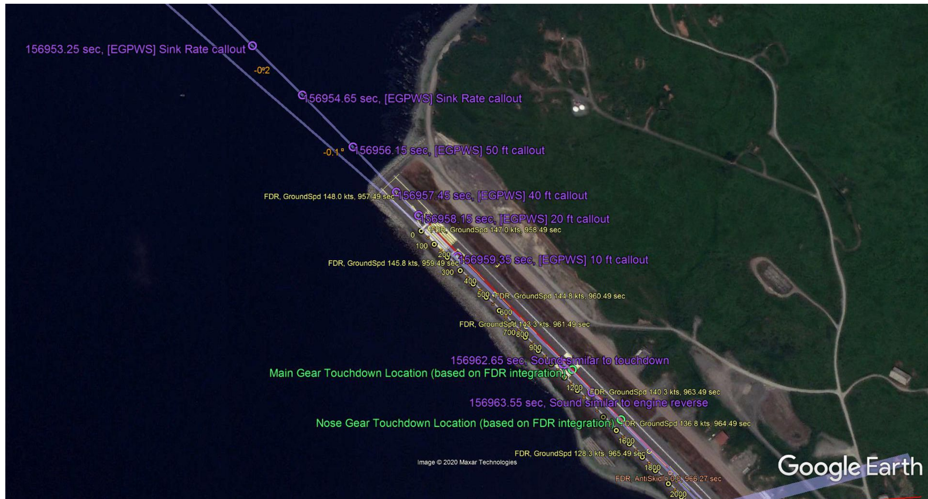
Figure A1.2: Planform view of runway 13 arrival end with N686PA sanitized CVR events (purple), FDR ground speed in knots (yellow), and FDR anti-skid fault parameters (orange, 1=fault) annotated along the airplane ground track. True north is toward the top of the page. The respective CVR and FDR time values represent FDR SRN and FDR SRN – 156000.
