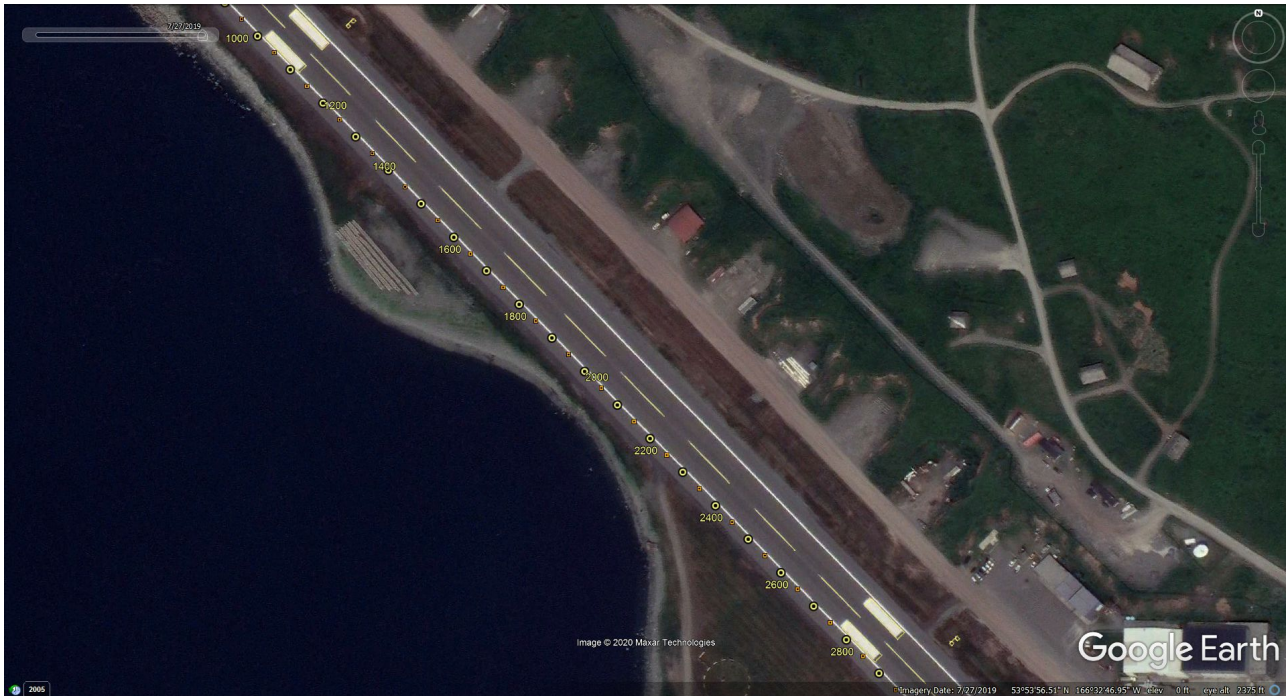
Figure 12: Google Earth model showing GPS survey of runway 13/31 midsection (solid yellow lines) including centerlines and the touchdown zone targets. True North is toward the top of the page.
