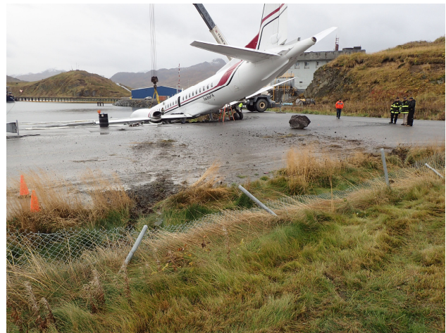
Figure 1(b): Airport perimeter fence, post and fence directional damage, displaced large rock and soil path across public roadway.
