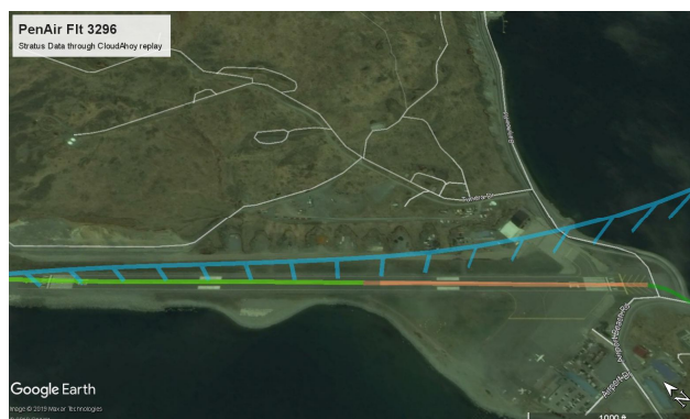
Figure 14(b): CloudAhoy reconstruction of N686PA flightpath during missed approach and landing rollout
