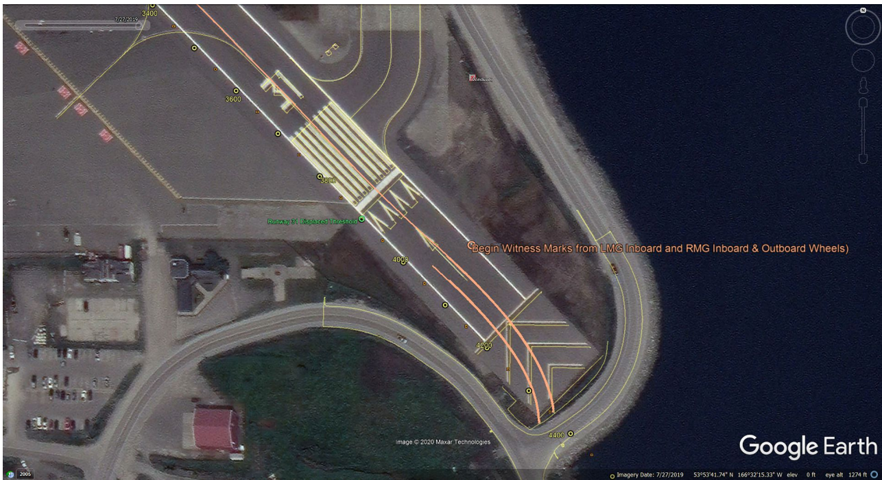
Figure 10: Google Earth model showing zoomed-in view of N686PA witness marks associated with the LMG inboard and outboard wheels and the RMG inboard and outboard wheels, as indicated by the respective solid orange lines. True North is toward the top of the page.
