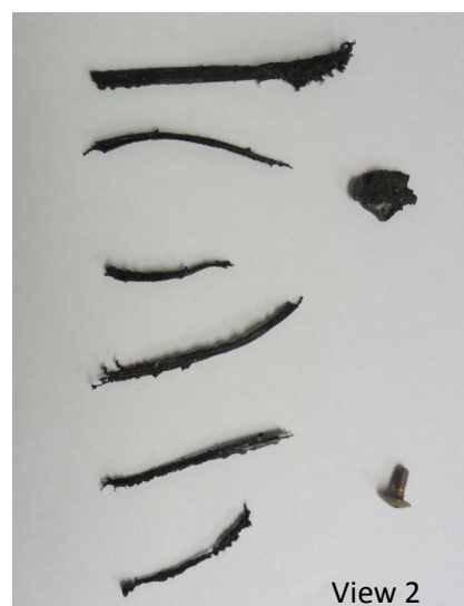
Figure 3: Tacky rubber strips, rubber piece, and screw (3/4 inch) recovered during runway 13 visual surveys
