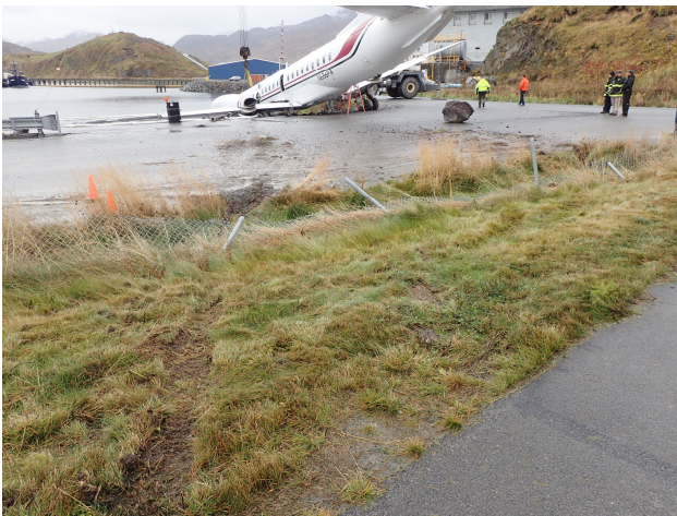
Figure 1(a): Left main gear wheel path exiting the blast pad surface, traveling across the grass, over the fence, across a ditch, and up on the roadway.
