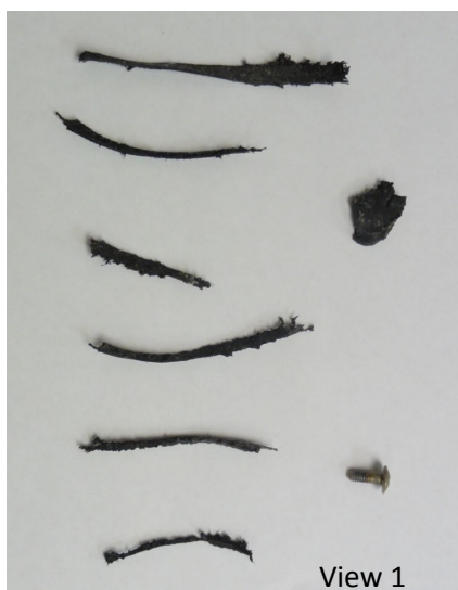
Figure 3: Tacky rubber strips, rubber piece, and screw (3/4 inch) recovered during runway 13 visual surveys
