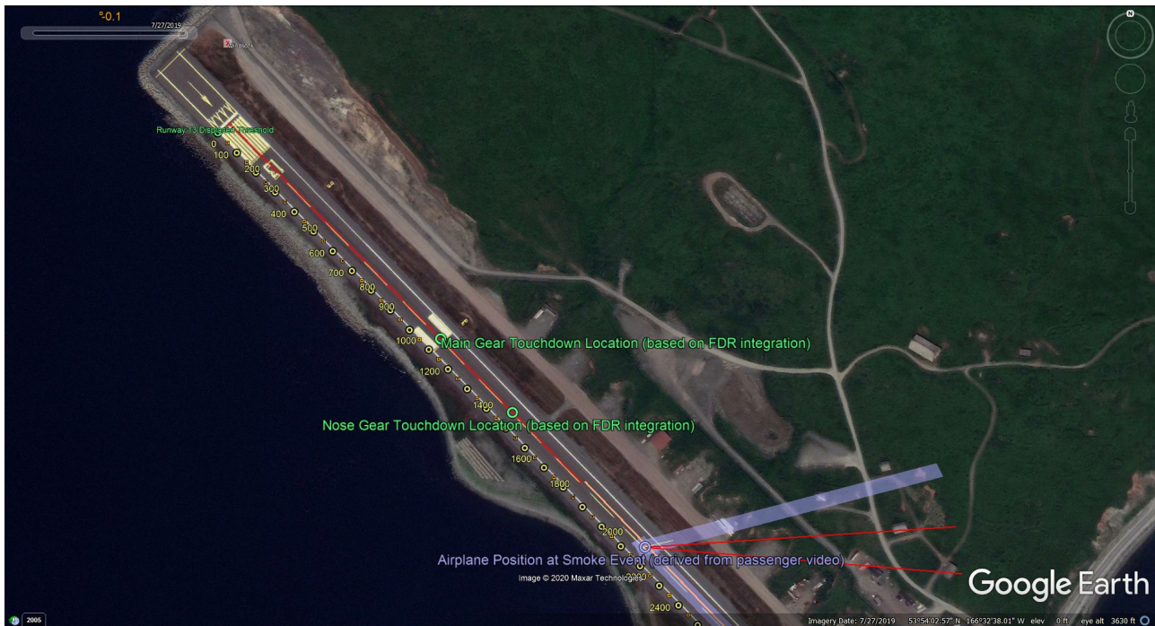
Figure 8: Google Earth model showing N686PA calculated gear touchdown points and GPS survey of ground rollout path on DUT runway 13. Witness marks associated with the LMG outboard wheel are highlighted in orange (beginning about 1,835 feet on the distance scale). True North is toward the top of the page.
