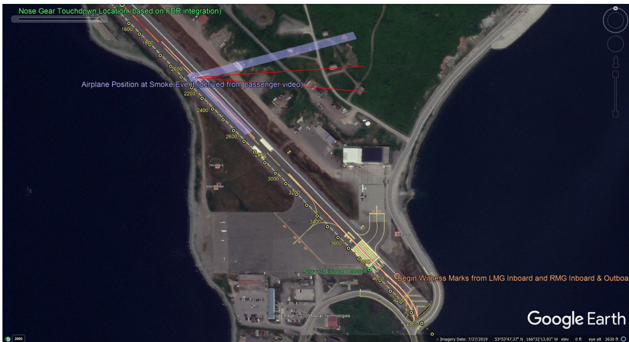
Figure 9: Google Earth model showing N686PA main gear wheel paths on DUT runway 13 based on GPS survey of witness mark evidence. Witness marks associated with the LMG inboard wheel and the RMG inboard and outboard wheels begin near the midpoint of the 300-foot declared distance RSA, as indicated by the respective solid orange lines. True North is toward the top of the page.
