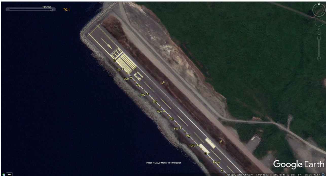
Figure 11: Google Earth model showing GPS survey of runway 13 arrival end markings (solid yellow lines) including arrows, threshold markings, runway number, centerline markings, and the touchdown zone target. True North is toward the top of the page.
