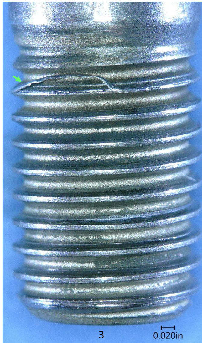
Figure 7 Close view of the threads from NAS6705-12 bolt 3 shown in Figure 4. The thread exhibited thread tip damage near the start of the grip (see green arrow).
