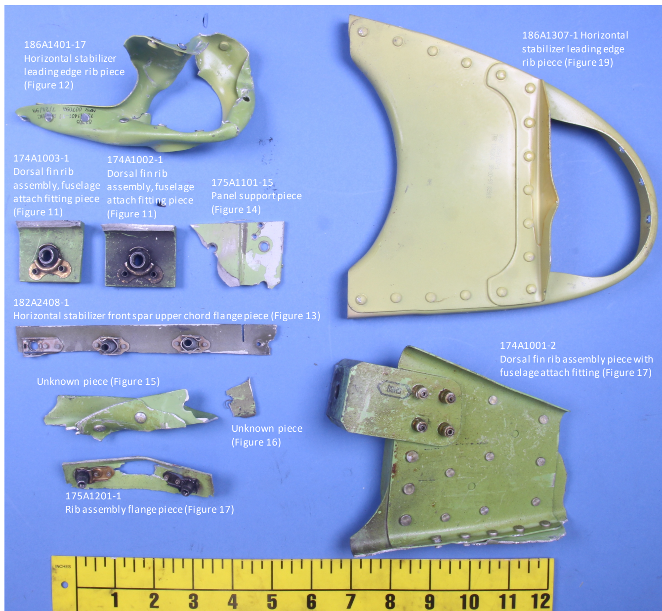
Figure 2 Image of the as-received structural pieces. Where known, Boeing part numbers are indicated.
