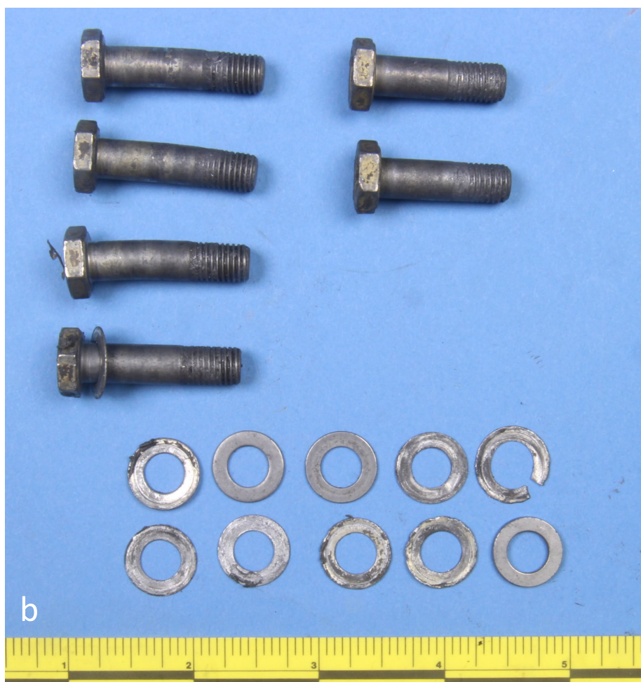
Figure 1 Image of the as-received bolts and washers. The bolts were not marked or identified relative to their installation locations.
