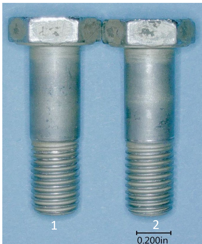
Figure 9 The NAS6705-09 bolts, after ultrasonic cleaning in acetone. Longitudinal view of the bolts.
