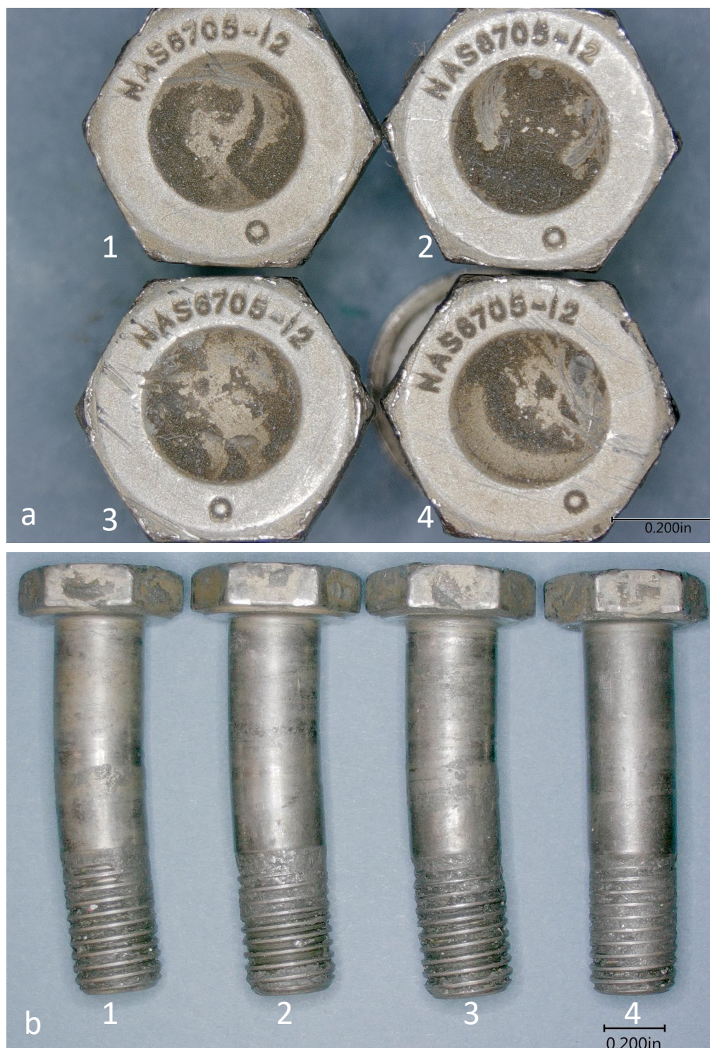
Figure 3 The NAS6705-12 bolts, as-received. The bolts were arbitrarily numbered for identification purposes. View (a) shows the bolt heads with markings. The dark deposits in the center of the heads is residual sealant. View (b) shows the longitudinal view of the bolts. Bolts 1,2, and 3, exhibited pronounced bending deformation. The threads are filled with anti-seize compound.
