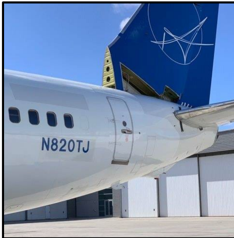
Figure 1-N820TJ missing dorsal fin and vertical stabilizer panels.
