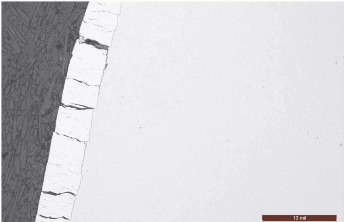
Figure 32 – BF optical micrograph of a closer view of the cracking in the chromium electroplated layer near the edge with the fracture surface (~100X, as-polished).
