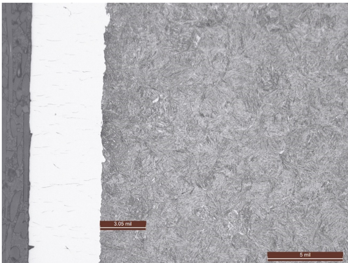
Figure 35 – BF optical micrograph of a closer view of the pin surface, showing the relative depth of the darker subsurface area (~500X, etched 2% Nital).
