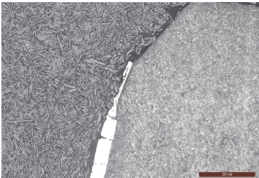
Figure 31 – BF optical micrograph of the location in Figure 30, after etching (~50X, etched 2% Nital).
