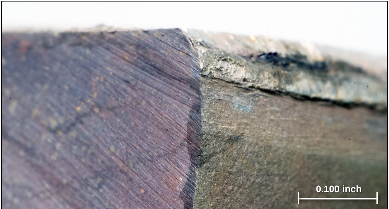
Figure 34 – The mating cross section to Figure 30, after chromium electroplated layer stripping.
