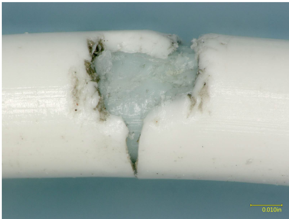
Figure 3: Damage to Wire W251-00059-22 (150x magnification)
