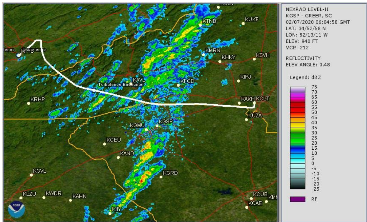
Figure 16 - KGSP WSR-88D 0.5° base reflectivity image for 0059 EST with the flight track
