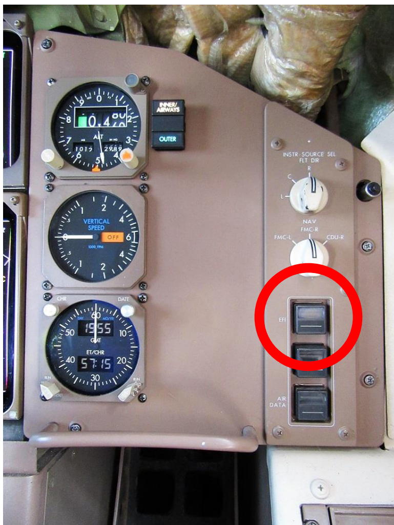
Photo 13: Photo showing Right Instrument Source Selector Panel (Lower) located on the right (FO) side of the forward control panel on the accident airplane (the EFI switch is indicated by the red circle). 159
