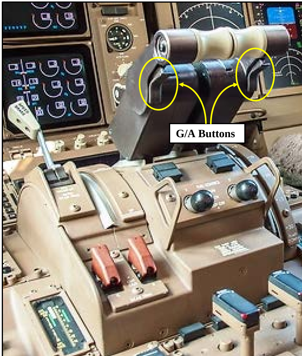
Figure 4: Representative B-767 Throttle Quadrant with G/A Buttons
