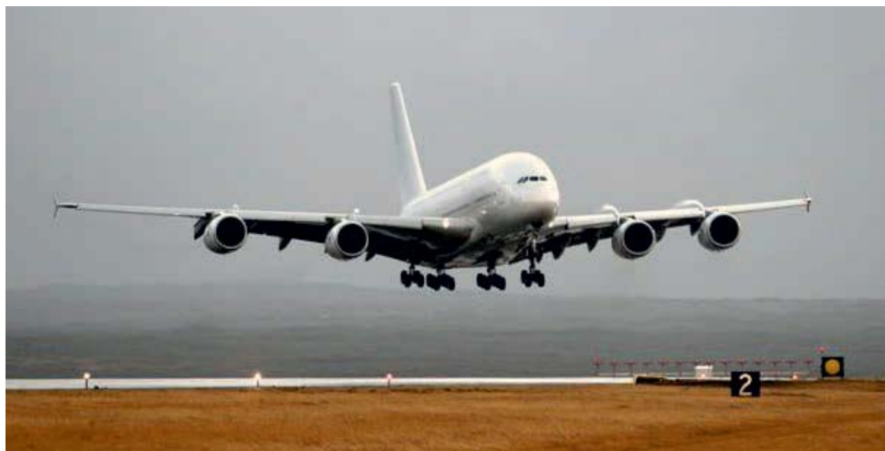
Figure 2 "Crabbed" final approach to Keflavik, Iceland. Picture taken from the south taxiway with the runway easily visible. Maximum reported crosswind at the time was 56 kt in gusts
