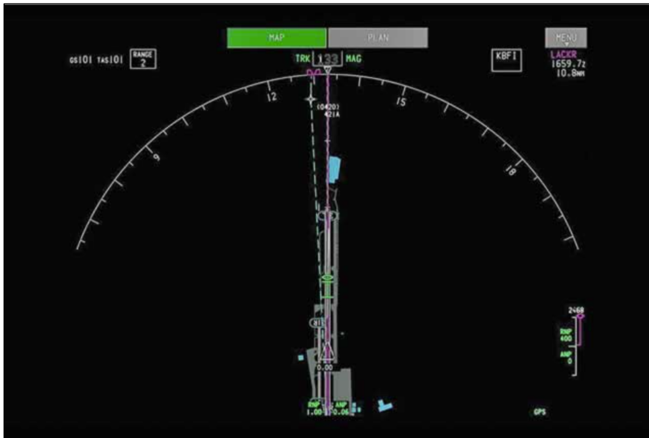
Figure 20. Boeing RAAS optimized runway exiting: Predicted (green bars) and actual (green oval) stopping performance displayed on an Airport Moving Map (from Reference 25).
