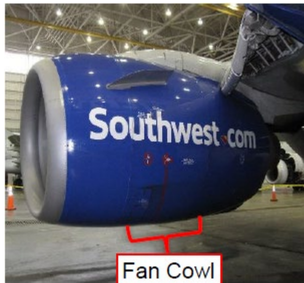
Fig. 5. Picture of CFM56-7B engine highlighting the fan cowl.
