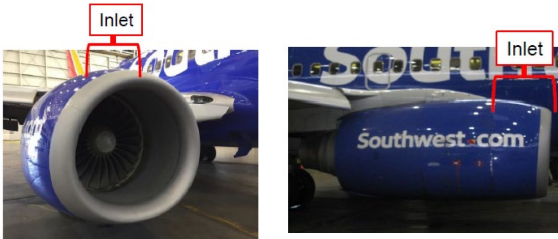
Fig. 1 and 2. Pictures of CFM56-7B engine highlighting inlet.
