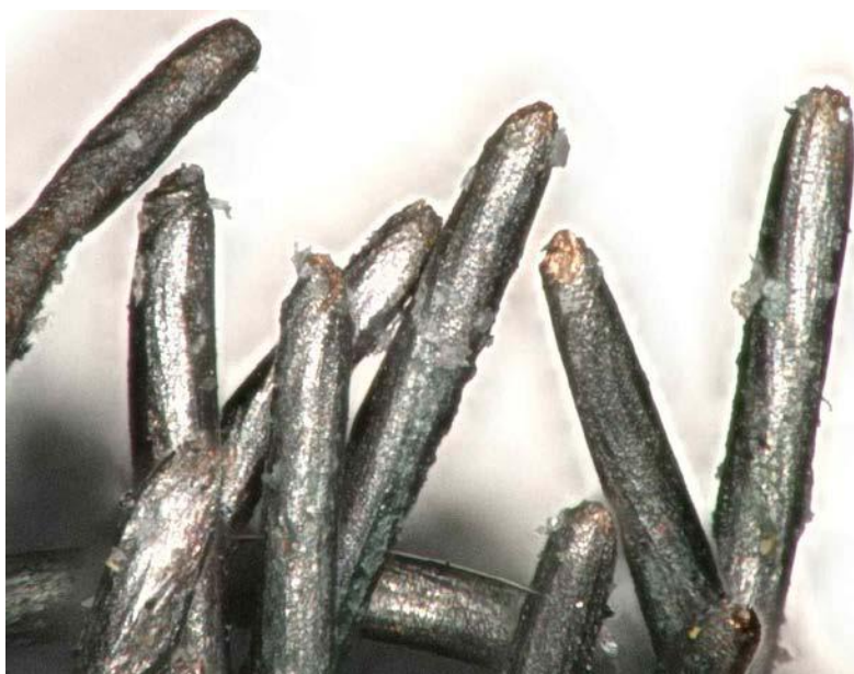
Figure 9: Fractured, individual wire strands at the ground wire termination point
