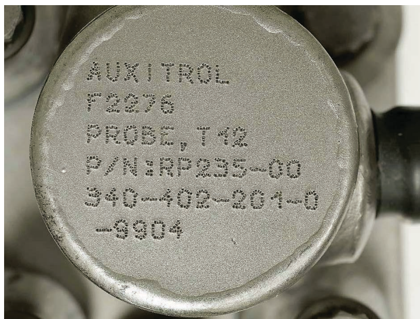
Figure 3: Data markings on T12 sensor
