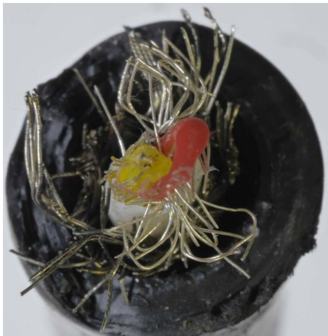
Figure 6: Fracture termination point of wire B
