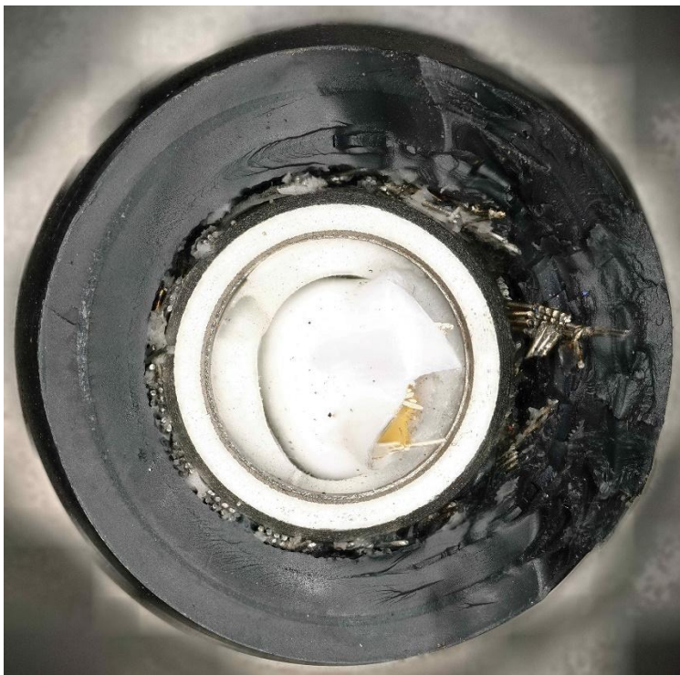
Figure 4: Fractured termination point of wire A
