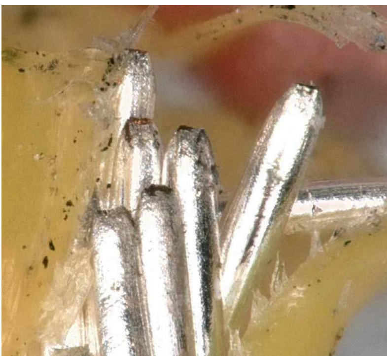
Figure 7: Fractured, individual wire strands at the wire B termination point
