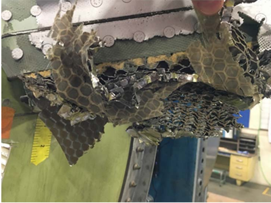
Figure 9-16 Crushed Honeycomb Attached to 9:00 Splice Plate, Inner Side
