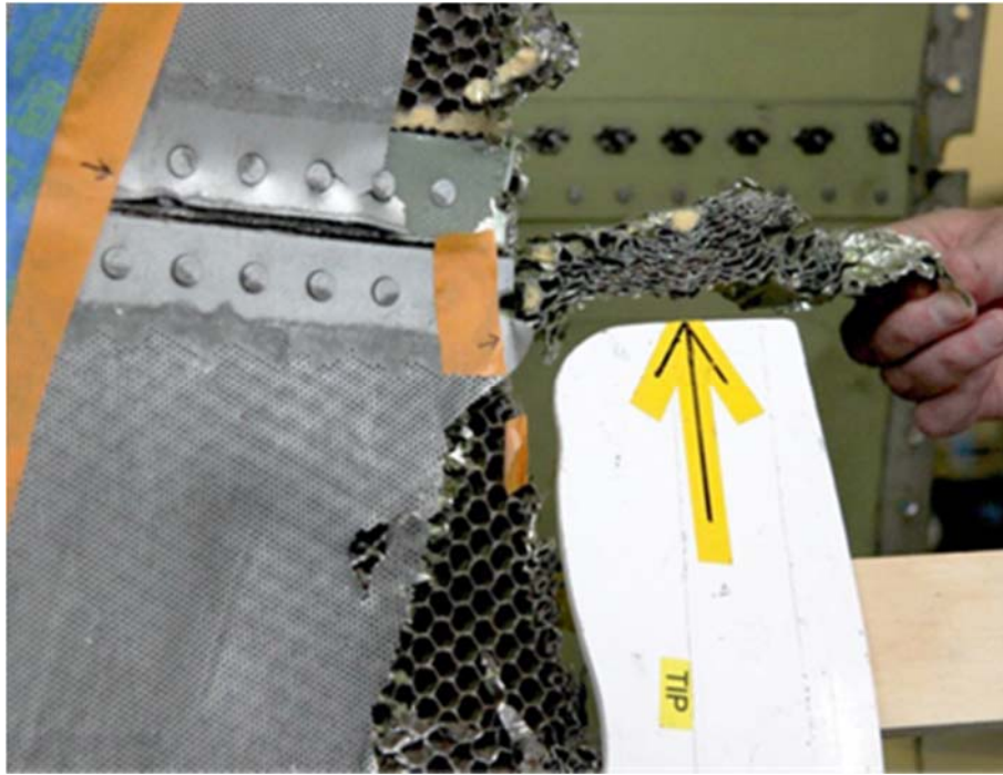
Figure 9-15 Recovered Honeycomb showing Direction of Crushing
