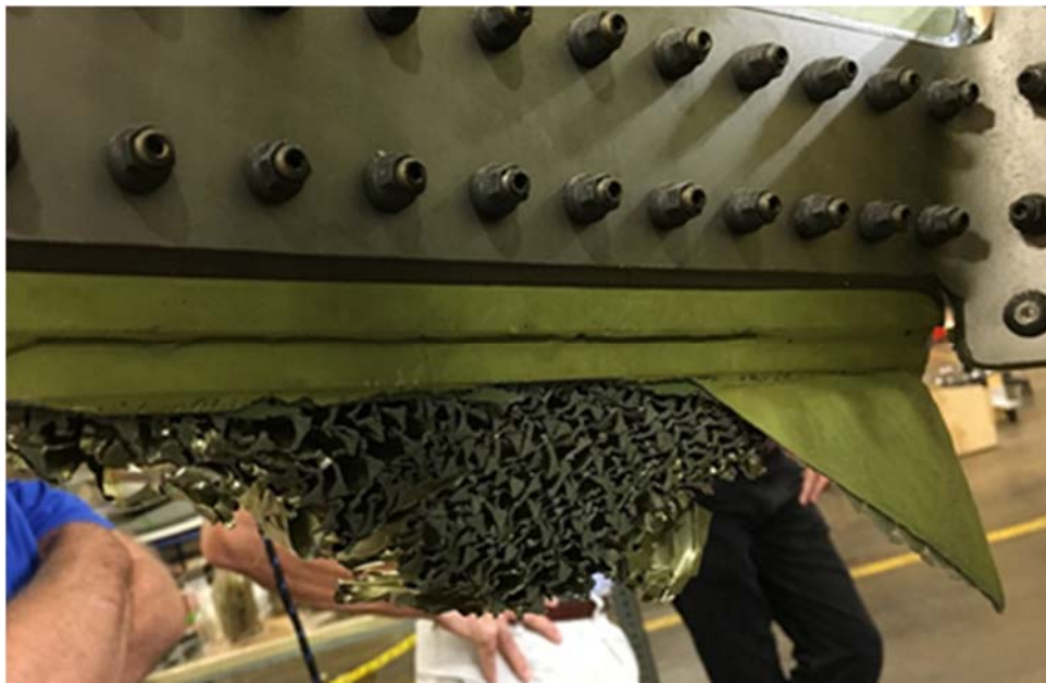
Figure 9-17 Crushed Honeycomb Attached to 9:00 Splice Plate, Outer Side
