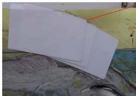
Figure 4-10 : Three distinct locations observed of the tip fragment trailing edge radius on Philadelphia engine 875134 Fan case
