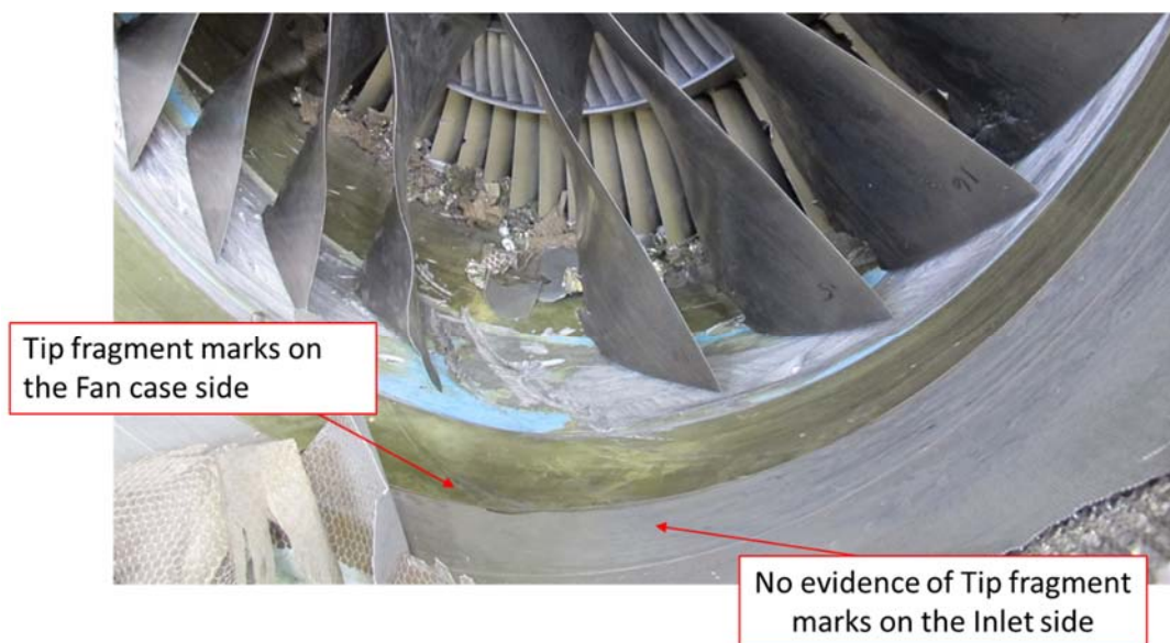
Figure 4-7 : Tip fragment marks on Philadelphia engine 875134
