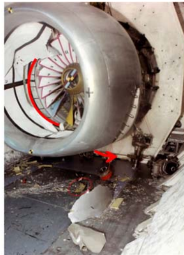
Tip panel exit through the inlet. Inlet still in place after FBO
