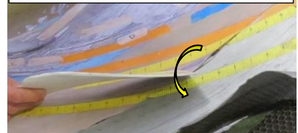
8) Tip's fractured-edge creates gouge scratches that change from \sim 30^\circ to \sim 20^\circ helix while tip rolls from sliding on fractured edge to sliding flat
