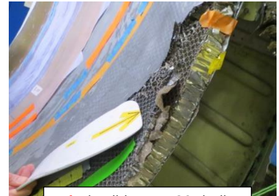
11) Tip slides at \sim 30^\circ helix delaminating perforate skin
