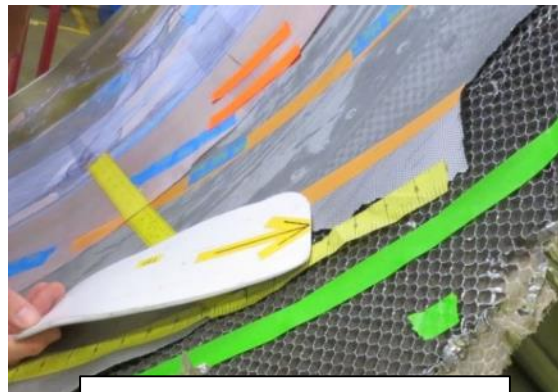
10) Tip slides at \sim 30^\circ helix delaminating perforate skin
