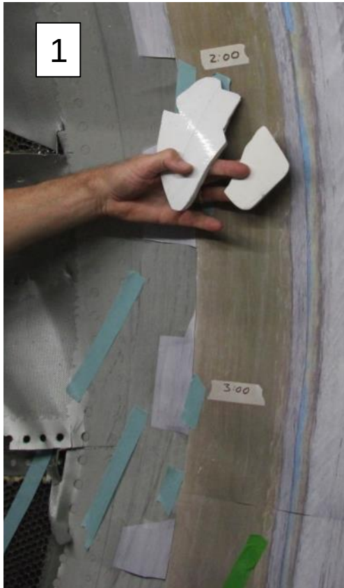
1), 2), 3) Additional fan fragments spiral into Inlet from 2:00 to 4:00 damaging perforate skin
