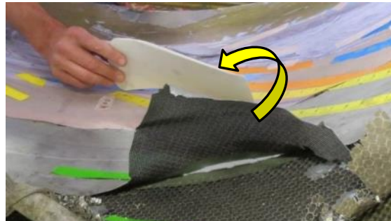
7) Tip rolls in reversed direction while its fractured-edge creates fan case scratches that begin with \sim 30^\circ helix
