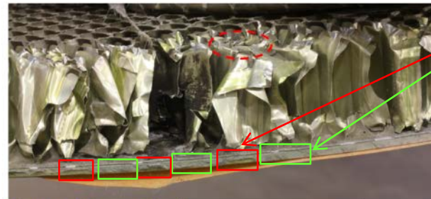
Titanium Alloy Particles Impacted and Imbedded
