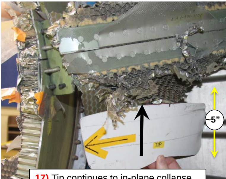
17) Tip continues to in-plane collapse ~5" of acoustic core into 9:00 beam
