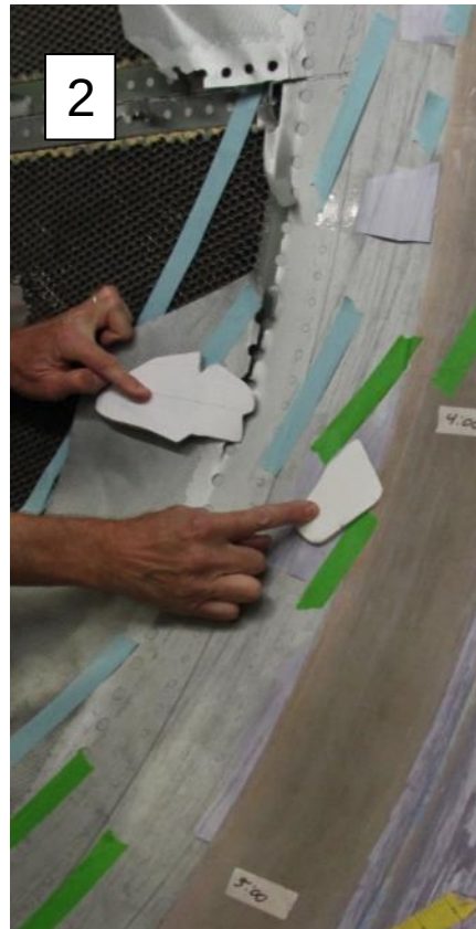
1), 2), 3) Additional fan fragments spiral into Inlet from 2:00 to 4:00 damaging perforate skin
