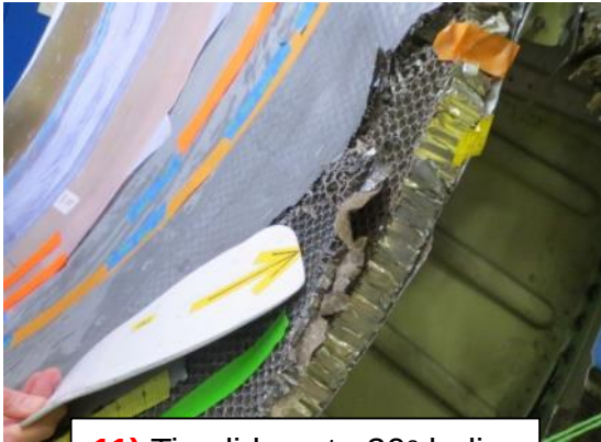
11) Tip slides at \sim 30^\circ helix delaminating perforate skin
