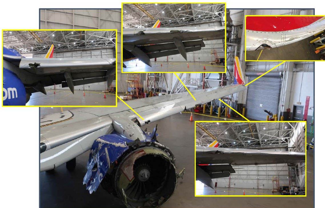
Figure 25 – Wing leading edge damage
