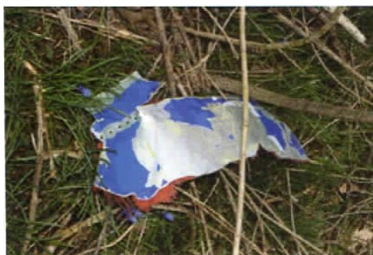
Figure 13 – Fan Cowl, Part 7 Site 1 (P7S1)
