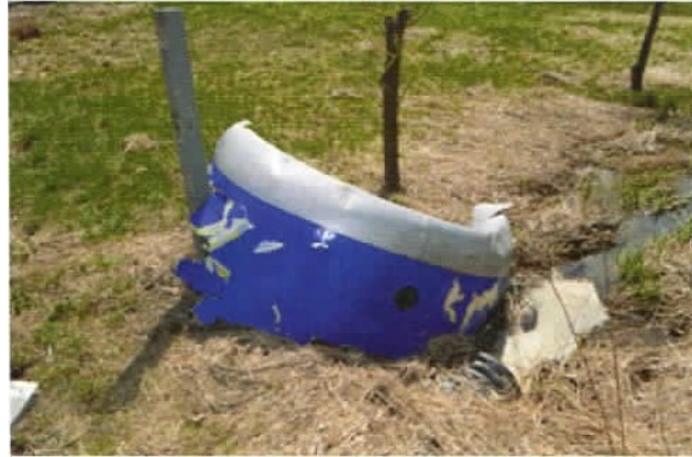
Figure 19 – Lower D-Duct and Outer Barrel, Part 1 Site 3 (P1S3)
