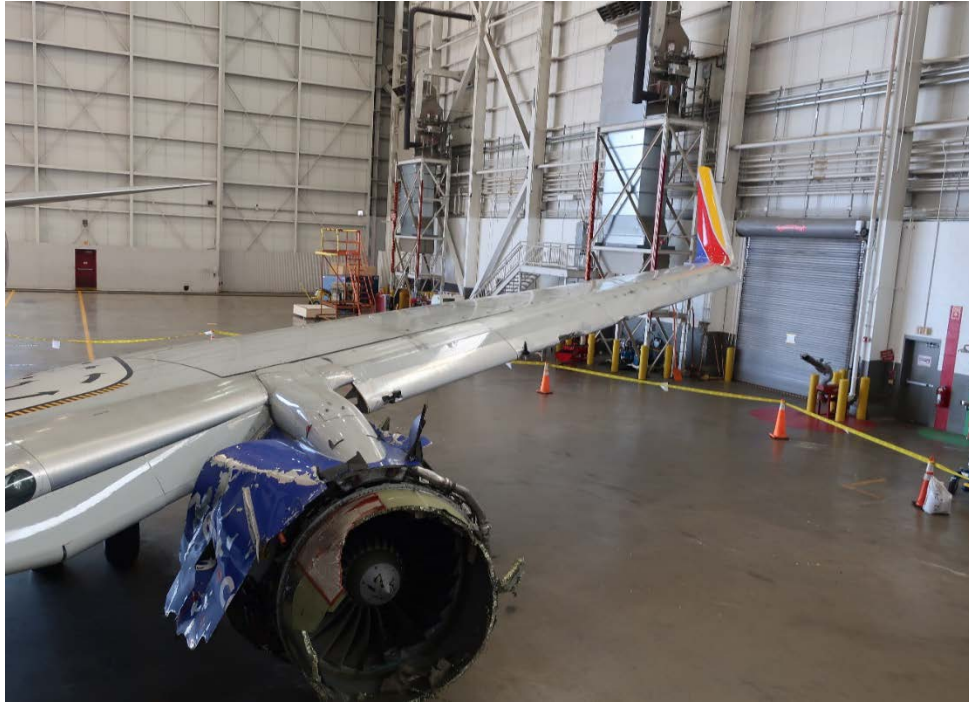
Figure 21 – Overview of wing and inlet damage
