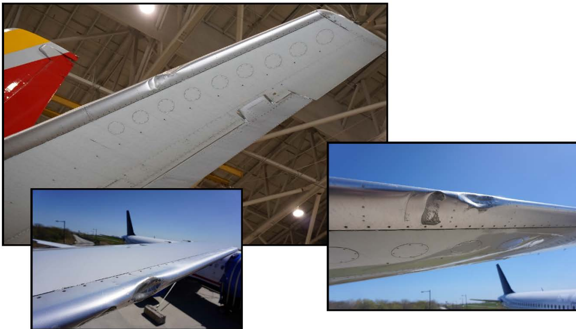
Figure 29 – Horizontal stabilizer damage
