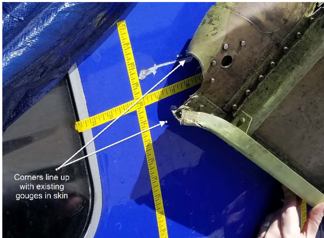
Figure 35 – Detailed witness mark comparison
