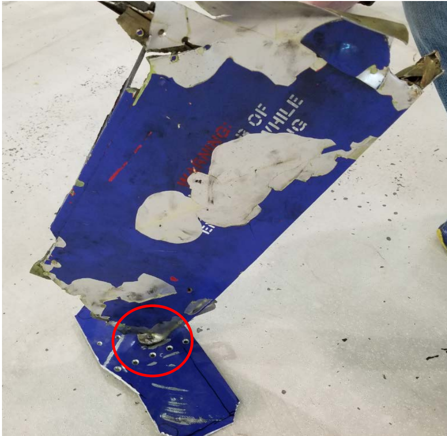
Figure 39 – Figure 38 impact damage to fan cowl section comparison
