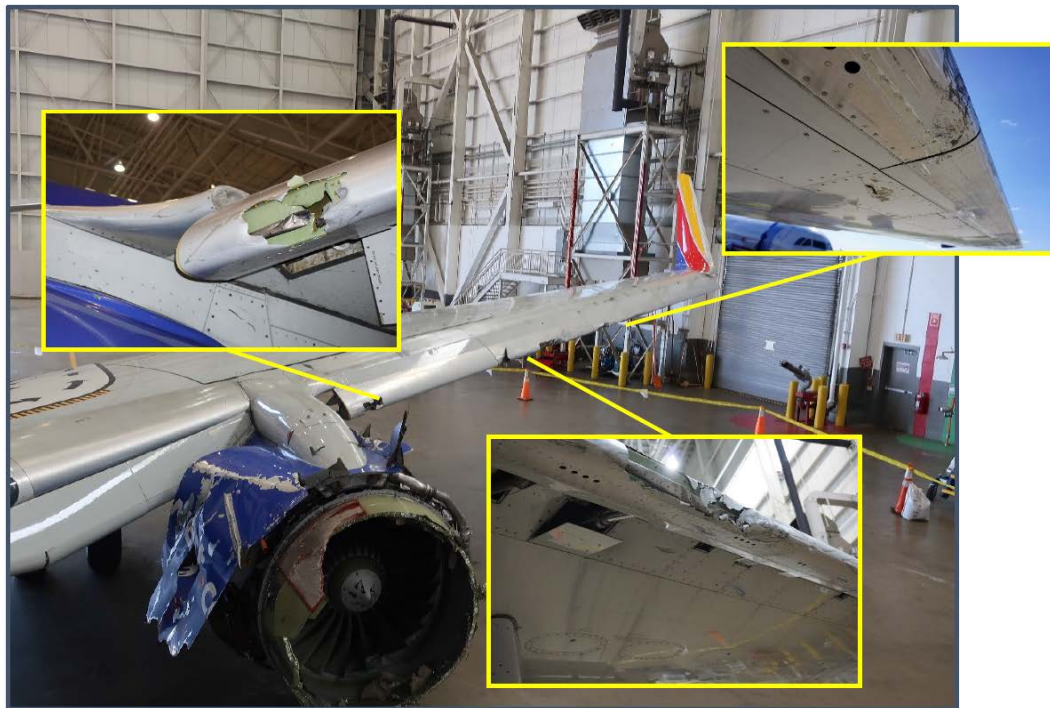
Figure 26 – Wing leading edge damage
