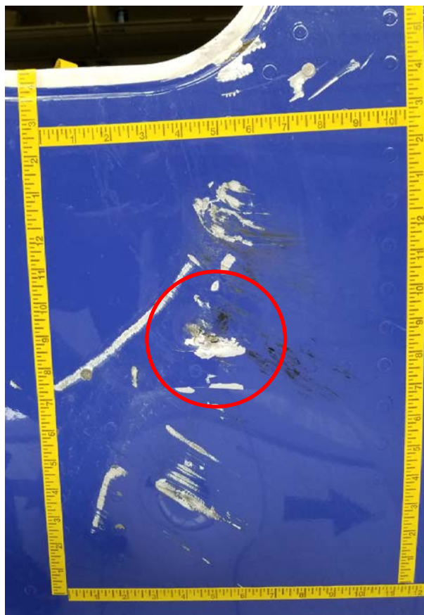
Figure 38 – Lower passenger window impact damage detail
