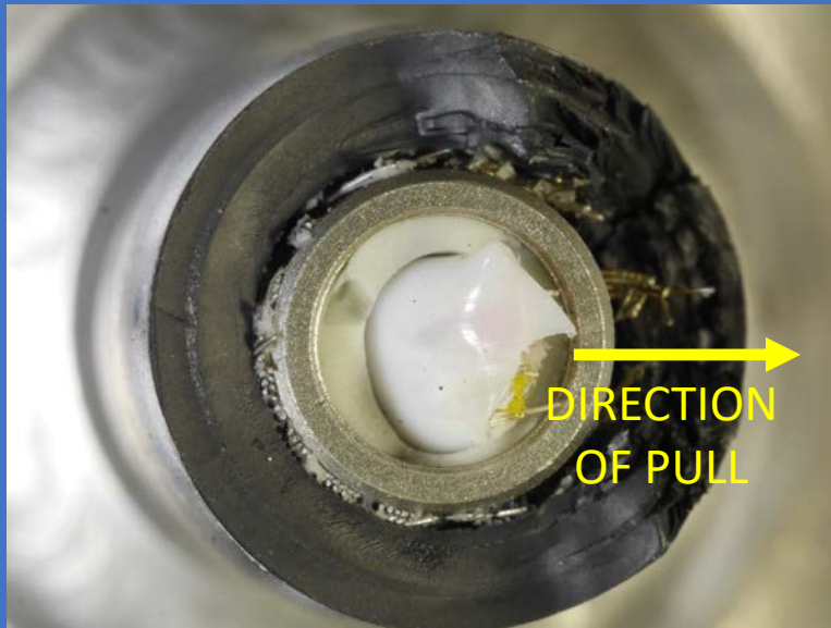
CHANNEL "A" FRACTURED AT PROBE
