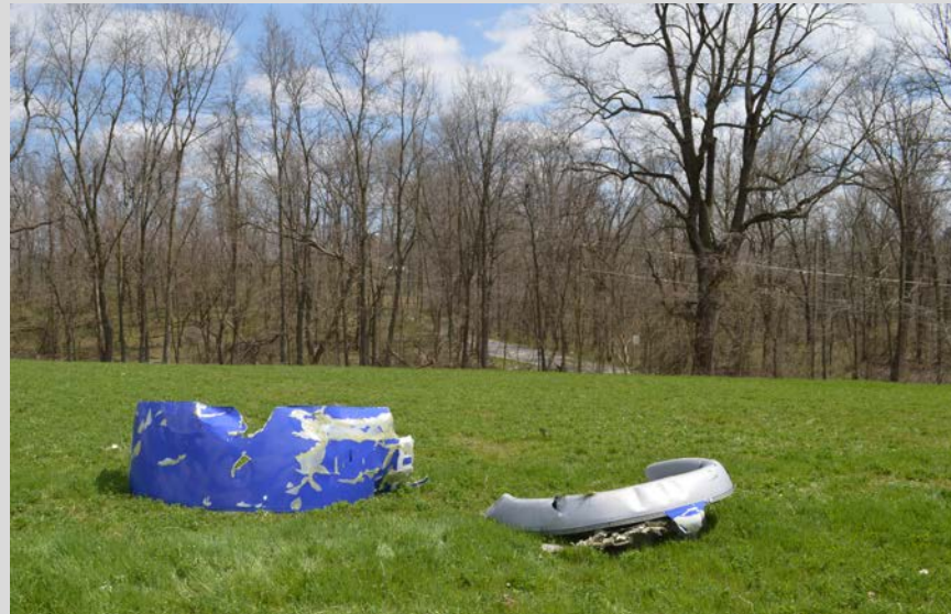
PHOTOGRAPH OF THE UPPER LIPSKIN AND OUTER BARREL IN A FIELD
