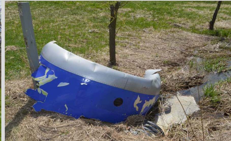
PHOTOGRAPH OF THE LOWER LIPSKIN AND OUTER BARREL IN A DITCH
