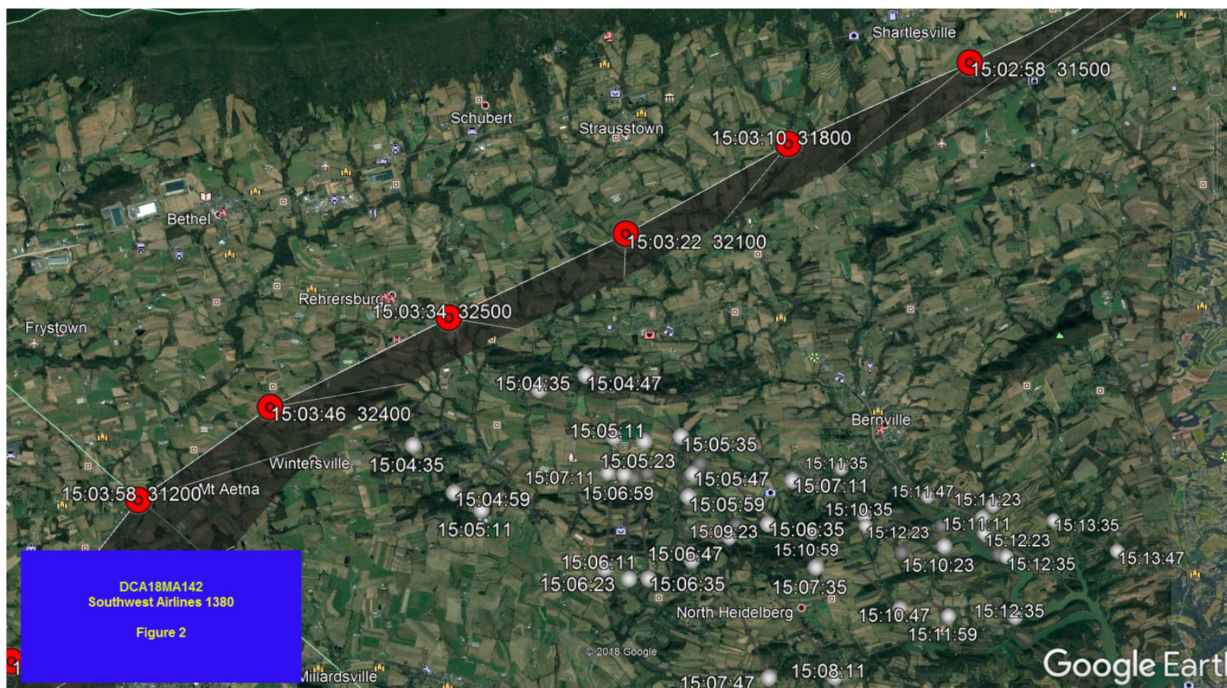
Figure 2 - Expanded view of the aircraft flight track indicating altitudes. The silver targets depict the primary targets moving away from the aircraft flight track.
