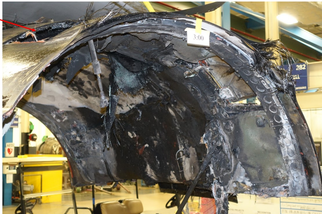
Photo 22- No. 2 Engine Right (Outboard) Thrust Reverser Door, Upper PRD Separated
