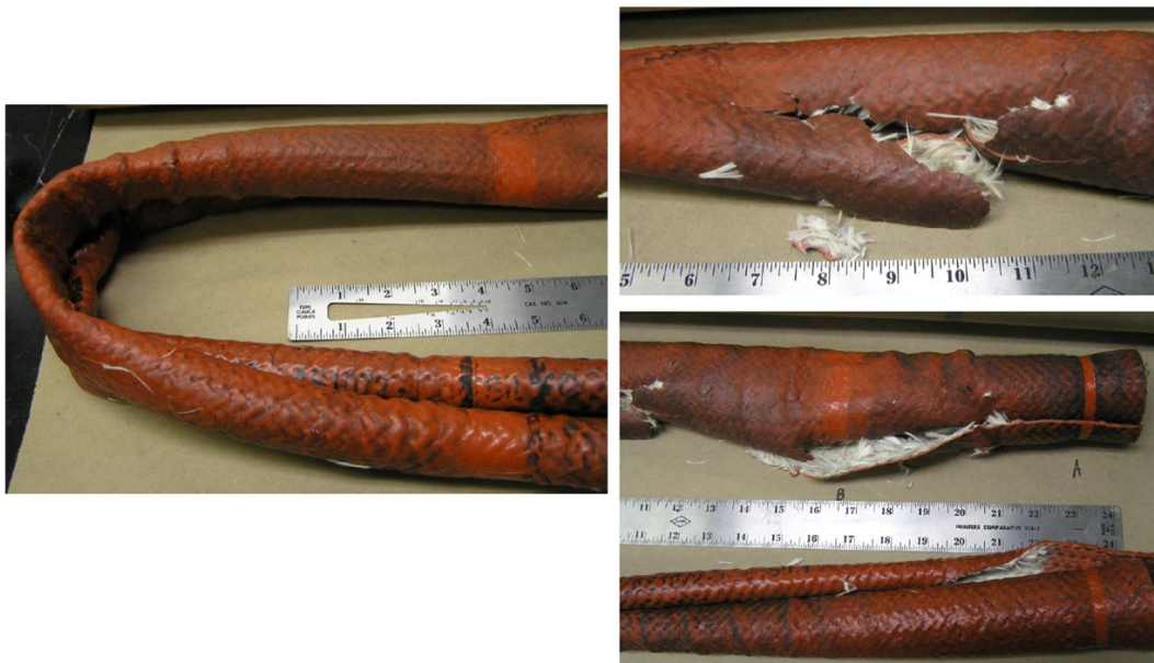
Photo 41- AMS FM-13 Hose Fire Sleeve, As Received at Parker Aerospace (Photos Courtesy of Parker)
