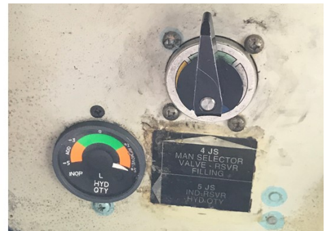
Photo 27- Hydraulic Service Panel (L) Yellow, (C) Green, (R) Blue
