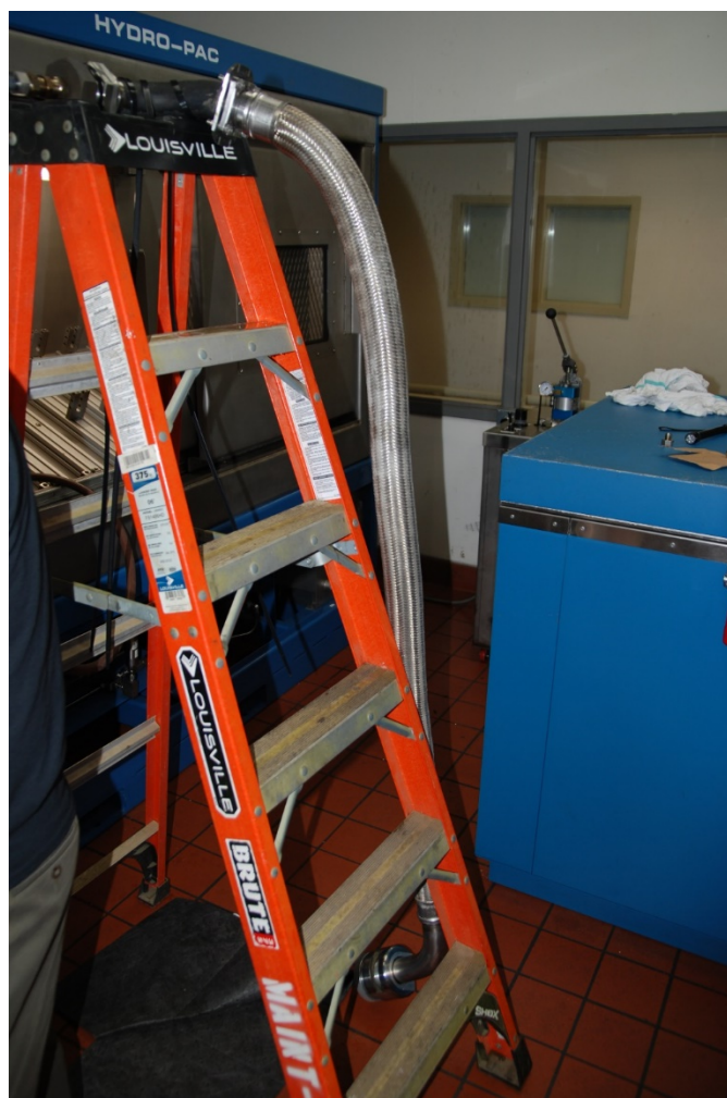
Photo 40- AMS FM-13 hose to Accident Rigid fuel pipe Flange Test Setup
