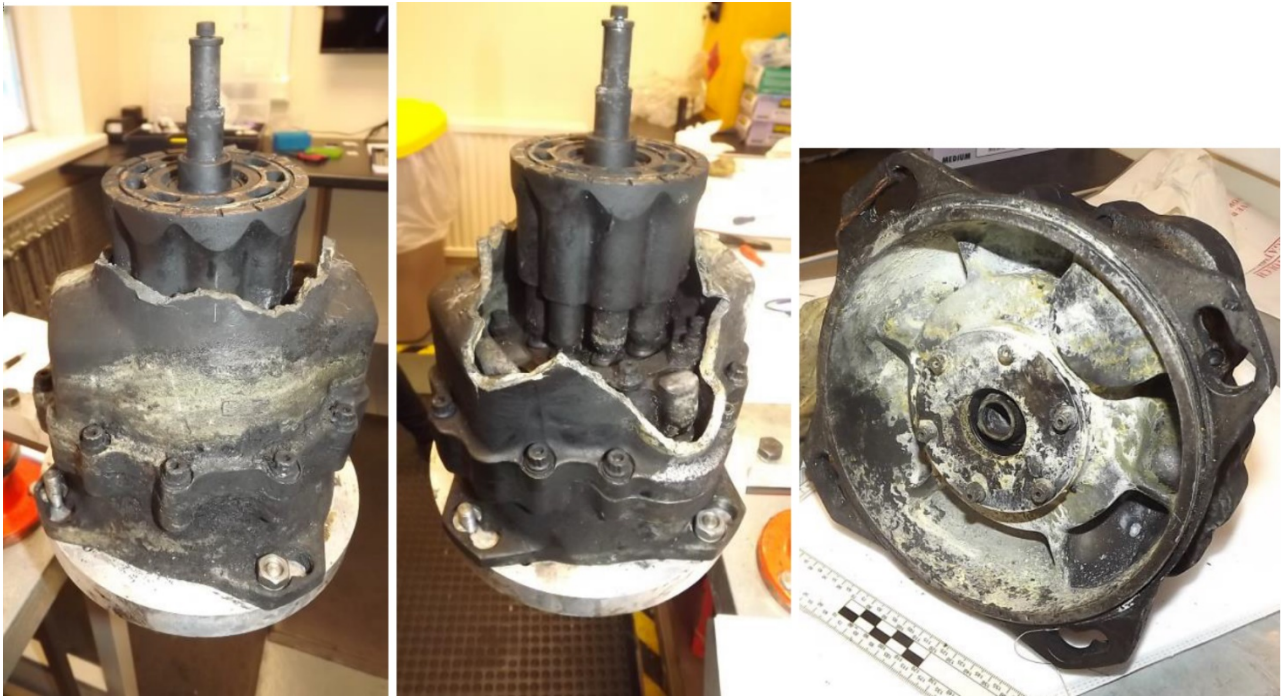
Photo 31- Yellow Hydraulic Engine Driven Pump, Bottom Section (Photos Courtesy of Eaton)
