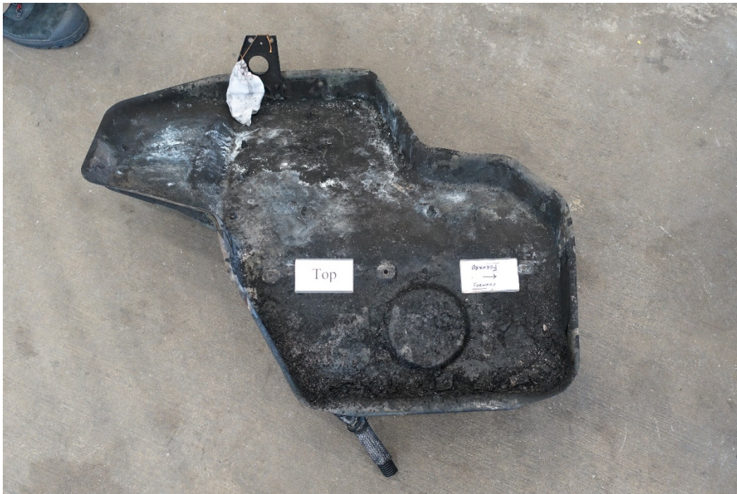
Photo 9- Fluid Drip Pan Located Under Pylon Hydraulic Interface Panel
