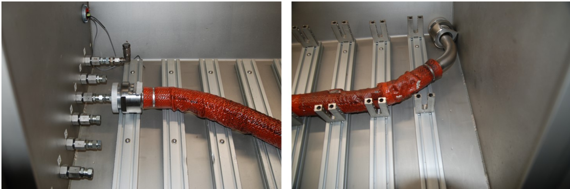
Photo 35- AMS FM-13 Hose in Pressure Test Bench
