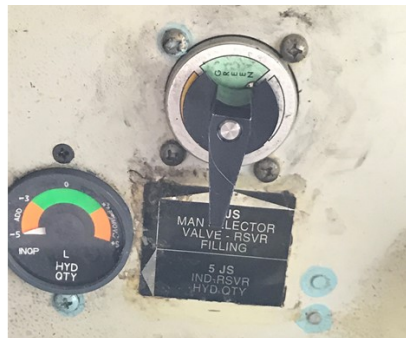
Photo 27- Hydraulic Service Panel (L) Yellow, (C) Green, (R) Blue
