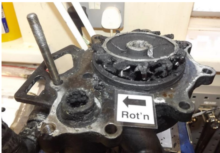
Photo 32- Yellow Hydraulic Engine Driven Pump Impeller (Photos Courtesy of Eaton)
