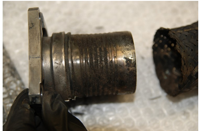
Photo 37- Accident FM-13 Hose Upper Flange Disassembly
