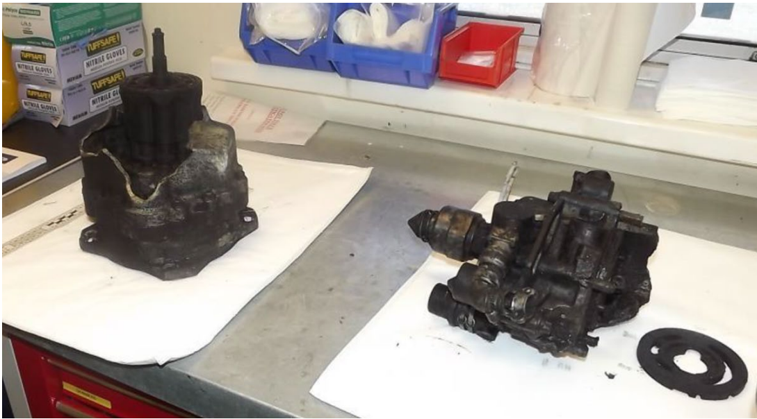
Photo 30- Yellow Hydraulic Engine Driven Pump, as Received at Eaton (Photo Courtesy of Eaton)
