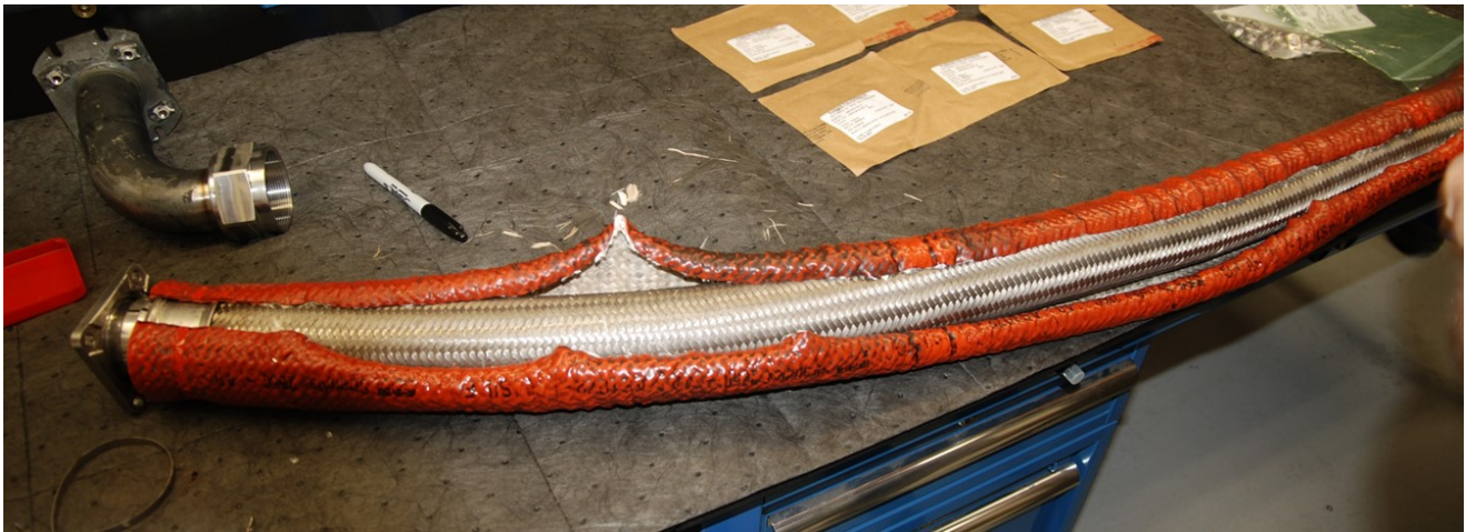
Photo 36- AMS FM-13 Hose Fire Sleeve Removal
