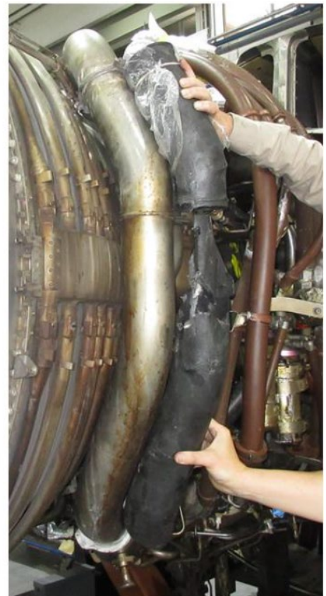
Photo 18- No. 2 Engine Starter Duct Damage, (L) Accident Engine, (R) Exemplar Engine (Photos Courtesy of Airbus)
