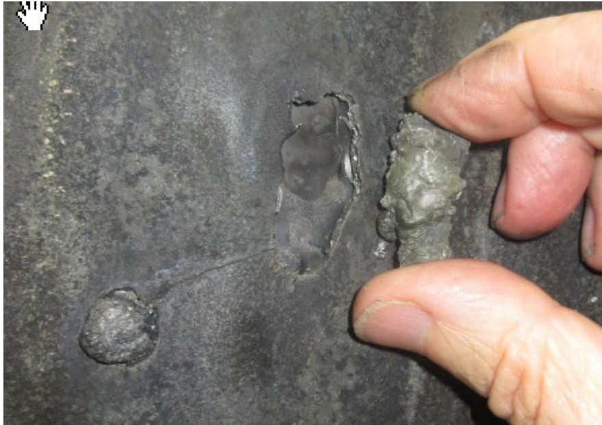
Photo 20- Photograph of Resolidified Metal Adhered to LPT Case (Photo Courtesy of Airbus)
