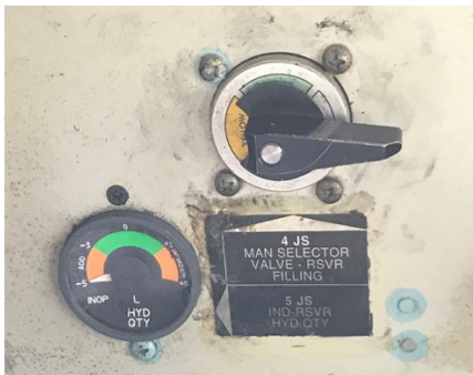
Photo 27- Hydraulic Service Panel (L) Yellow, (C) Green, (R) Blue
