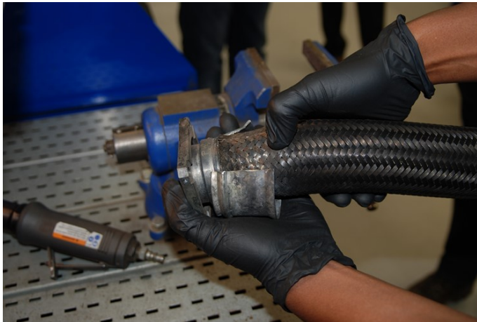
Photo 37- Accident FM-13 Hose Upper Flange Disassembly
