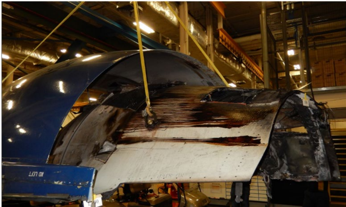
Photo 21- No. 2 Engine Right (Outboard) Thrust Reverser Door IFS
