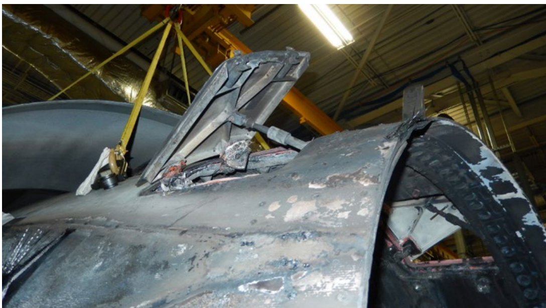
Photo 24- No. 2 Engine Left Thrust Reverser Door, Upper and Lower PRDs Open
