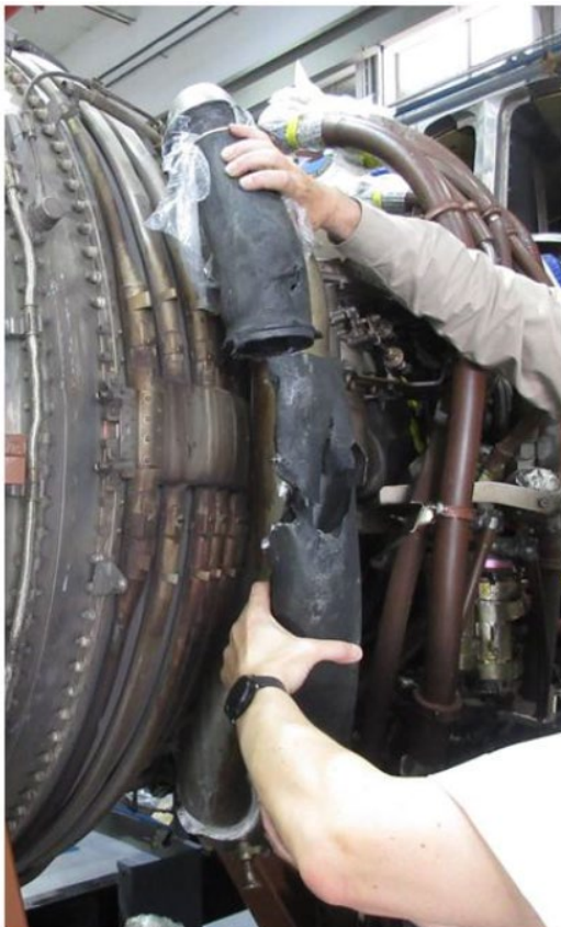
Photo 18- No. 2 Engine Starter Duct Damage, (L) Accident Engine, (R) Exemplar Engine (Photos Courtesy of Airbus)
