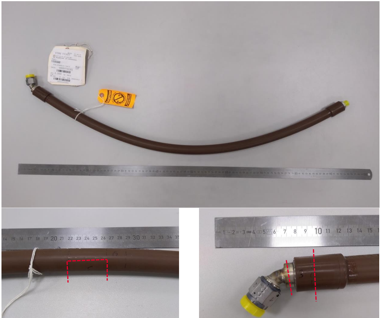
Figure 11 – visual inspection of a new hydraulic flexible hose.
