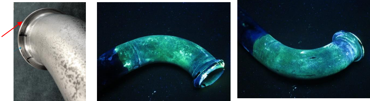
Figure 48: Penetrant inspection of pylon fuel rigid pipe pylon end without finding Conclusion: Following the NDT inspection no findings have been recorded.
