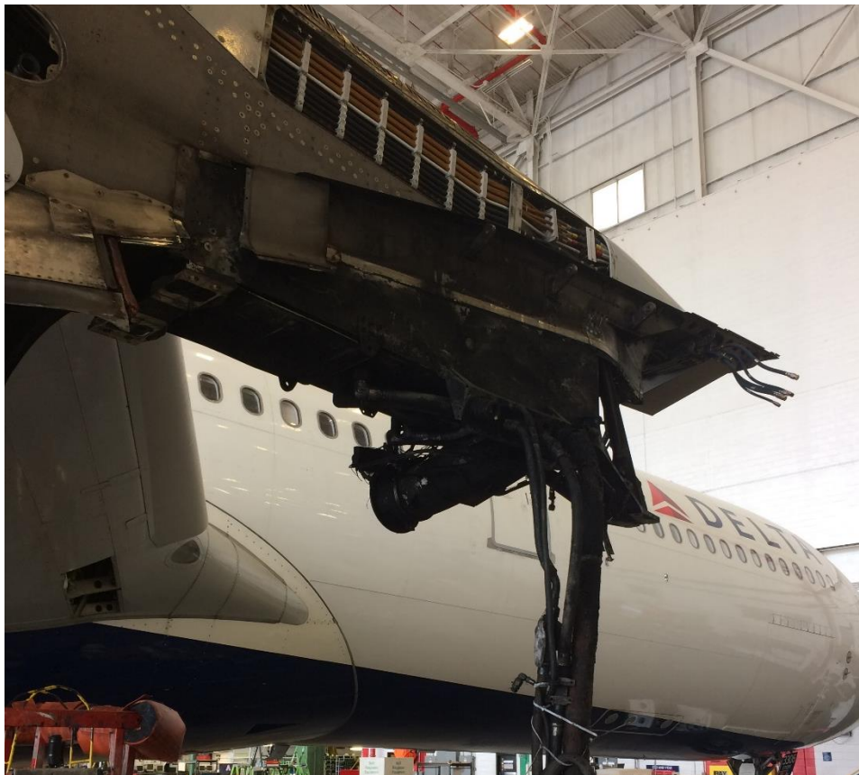
Figure 1: Overview of pylon area after removal of the affected engine
