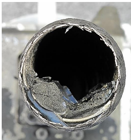
Figure 15: Flex line view in inboard direction presenting melted material on bottom side, at cut location
