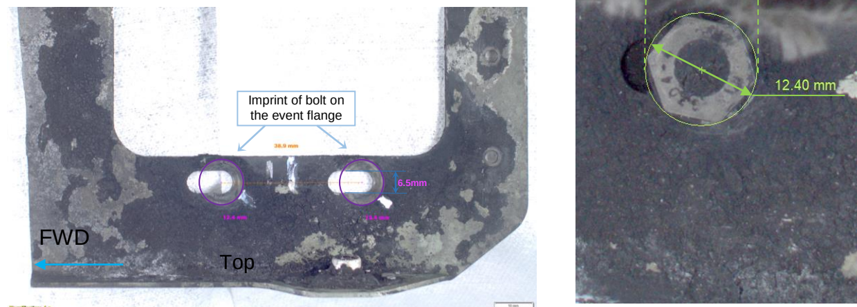
Figure 46: Face B- Fuel/hydraulic disconnect panel bolt measurements
