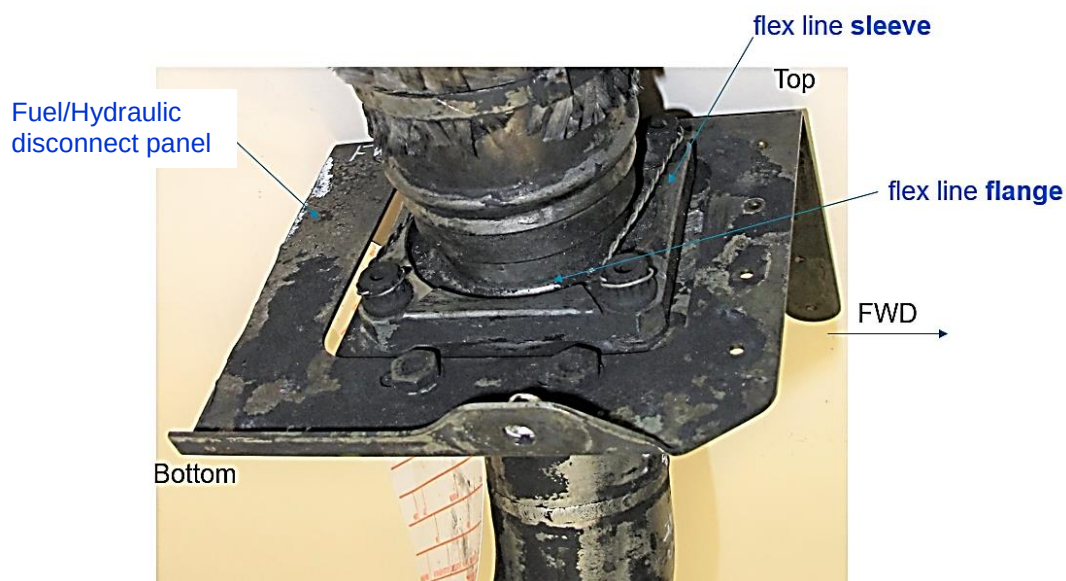
Figure 12: View from OTB (outboard) side - flex line sleeve and flange position to the fuel/hydraulic disconnect panel – no contact between sleeve and fuel/hydraulic disconnect panel
