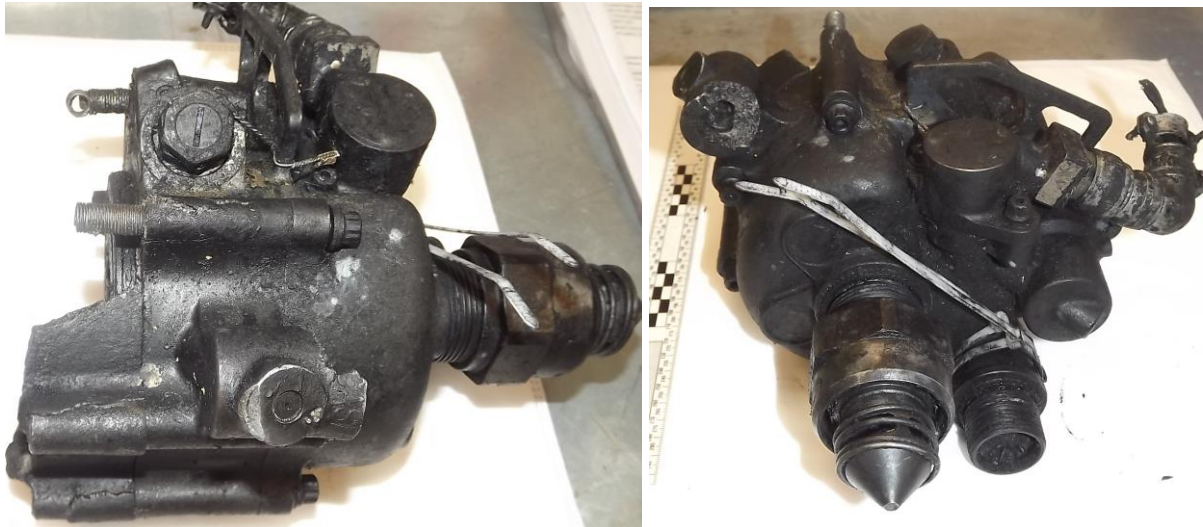
Photo No 5A and 5B: Valve Block External Surfaces
