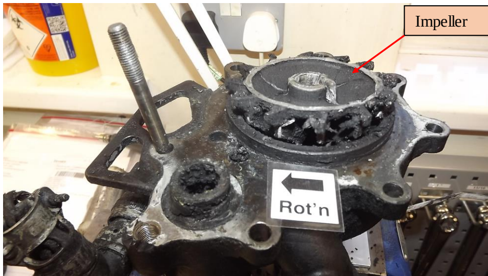
Photo No 13A : Impeller Retained in Adaptor Block
