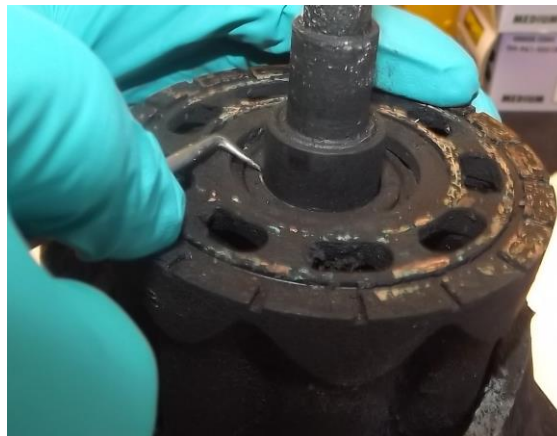
Photo No 7 : Alignment Mark Cylinder Block to Driveshaft
