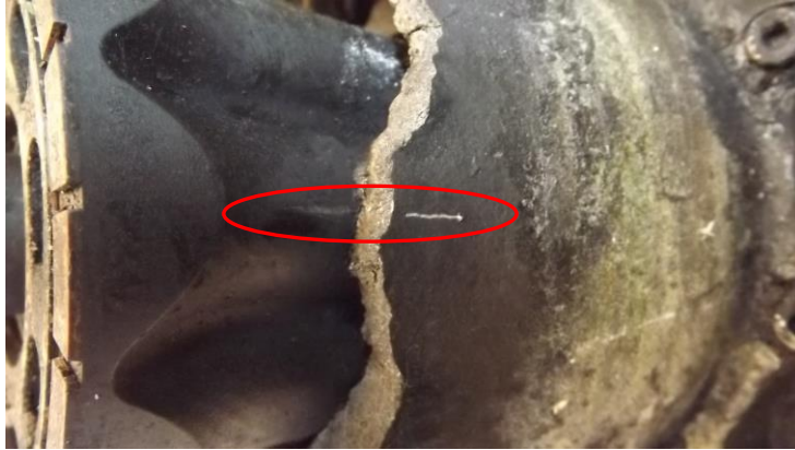
Photo No 8 : Alignment Mark Cylinder Block to Housing
