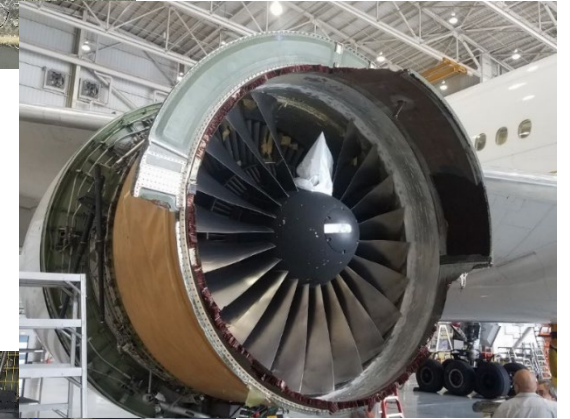
Fan Blade Impact Damage and Witness Marks
