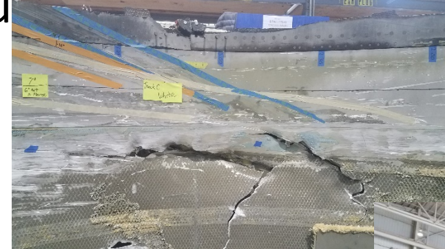
Fan Blade Impact Damage and Witness Marks
