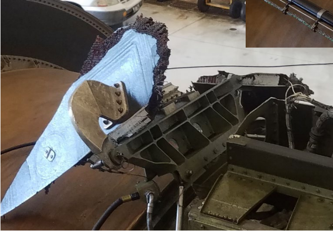
Fan Cowl Support Beam Fitting Attached to Fan Case
