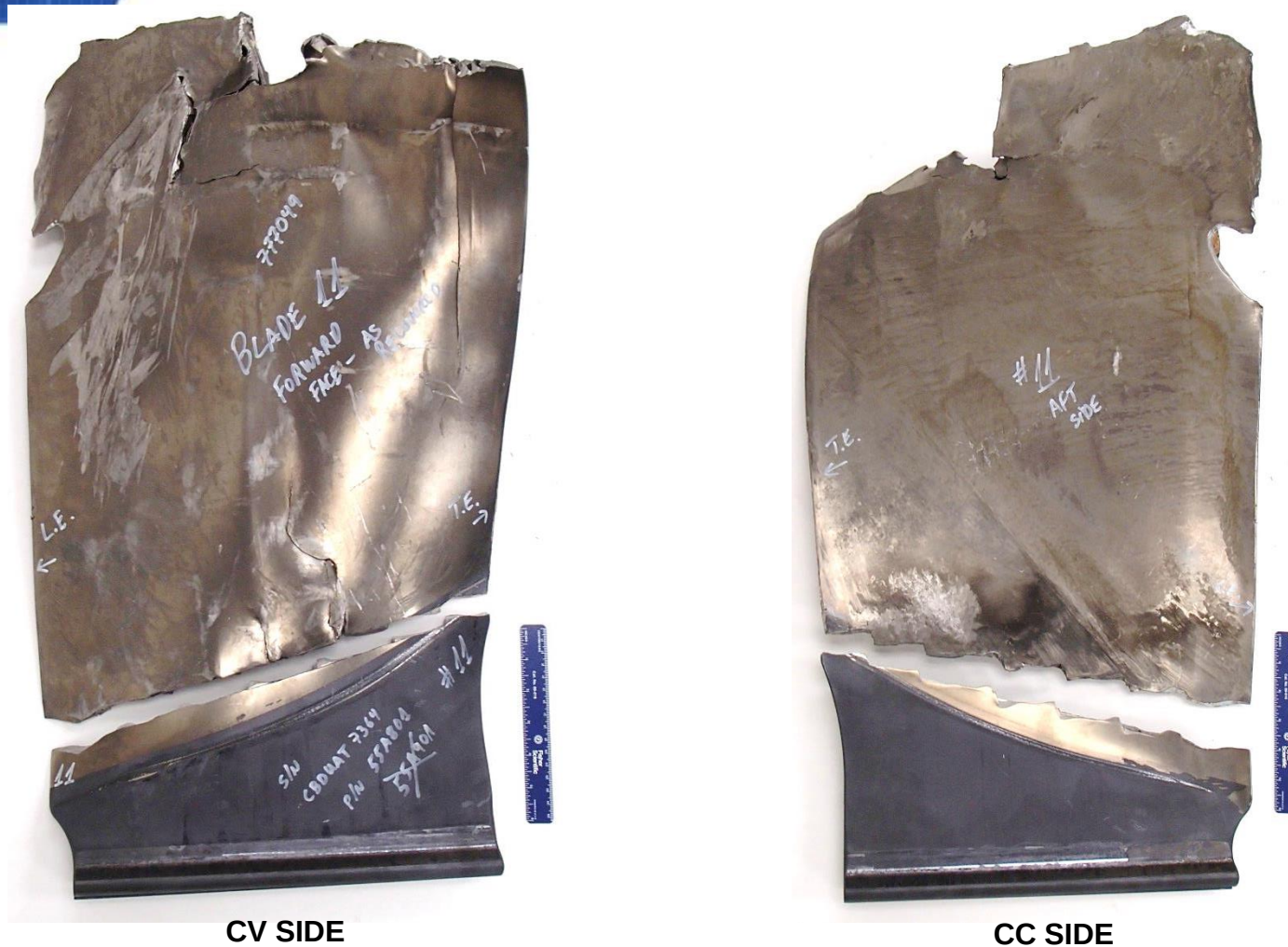
Figure 1 - Overall views of primary fractured Blade #11. Attachment 1
