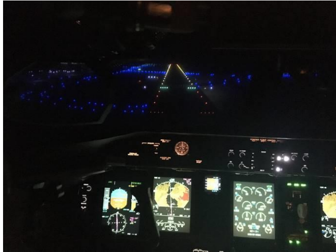
Photo 22: Run 3 runway lights at 150 feet agl.
