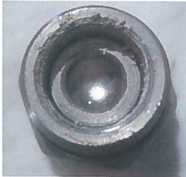
Photograph 8 – Rupture Disk Assembly.
