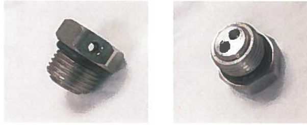
Photograph 5 – Rupture Disk Assembly.
