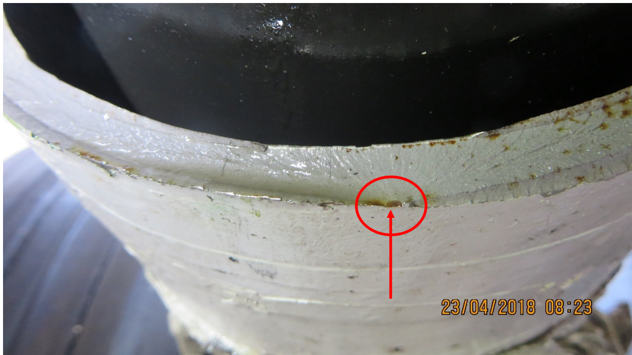
Figure 9 – Lower cylinder fatigue crack initiation site (forward side).
