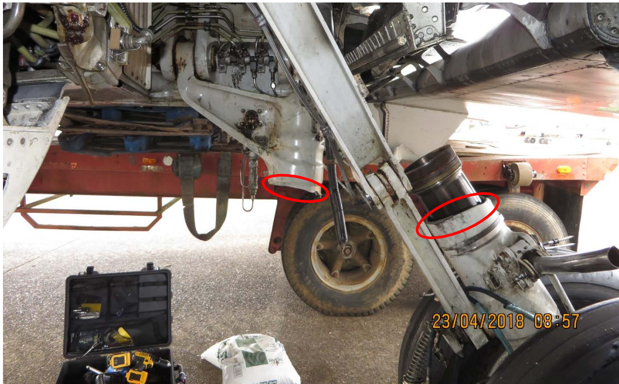
Figure 4 – Right main landing gear fracture looking outboard.
