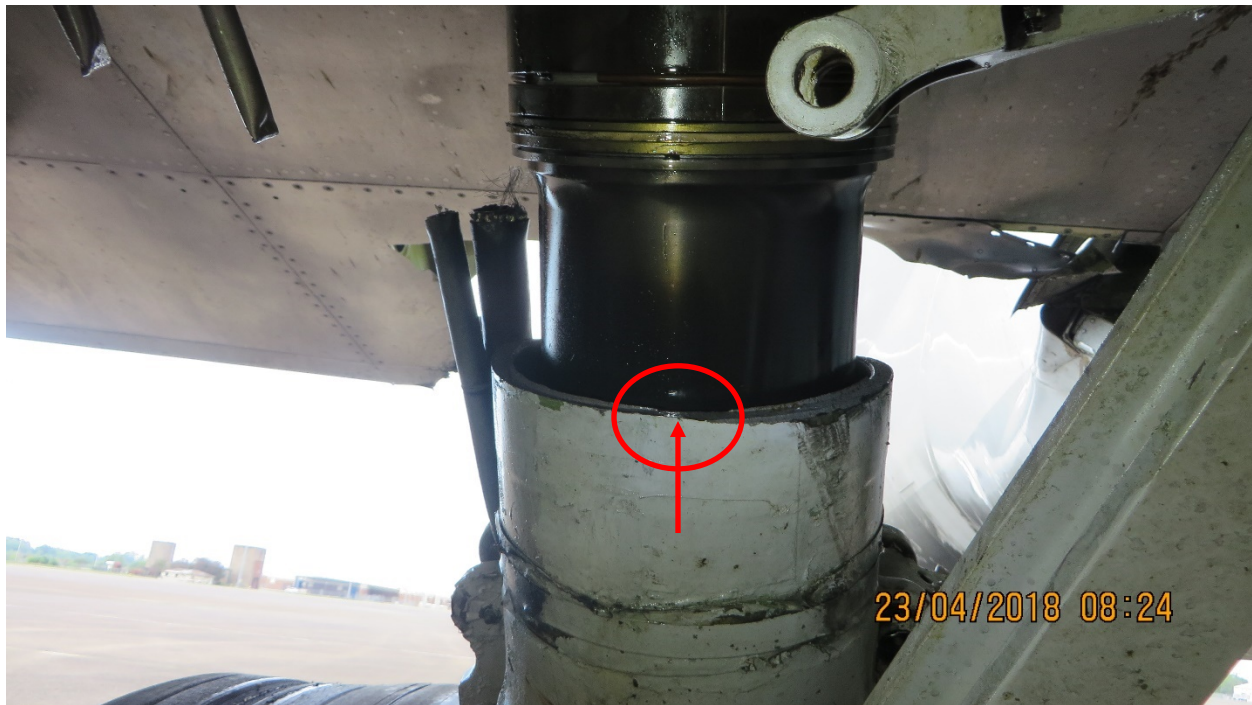
Figure 8 – Approximate fatigue crack initiation site on the lower cylinder (forward side).
