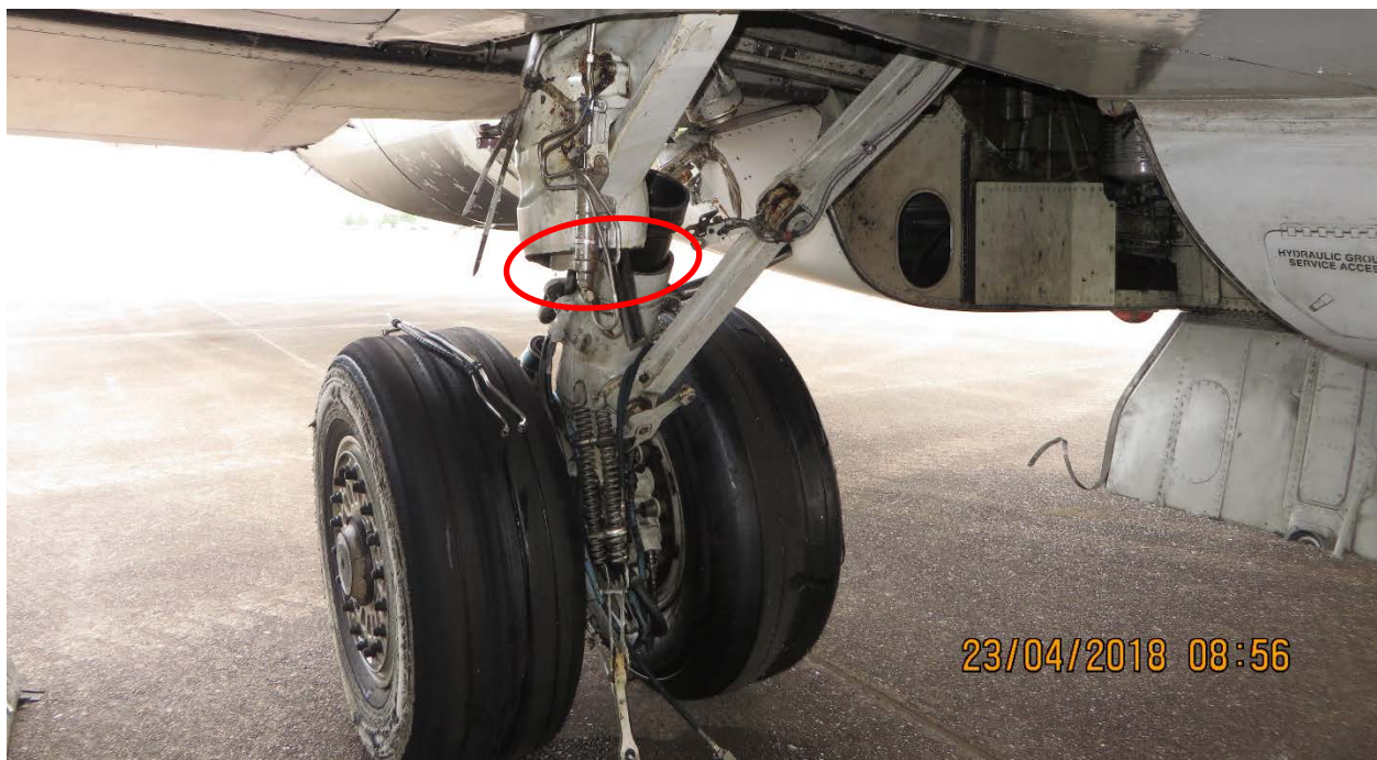
Figure 1 – Right main landing gear fracture looking aft and inboard.
