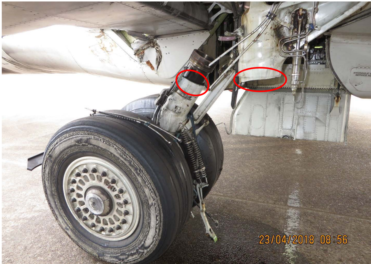
Figure 2 – Right main landing gear fracture looking inboard.
