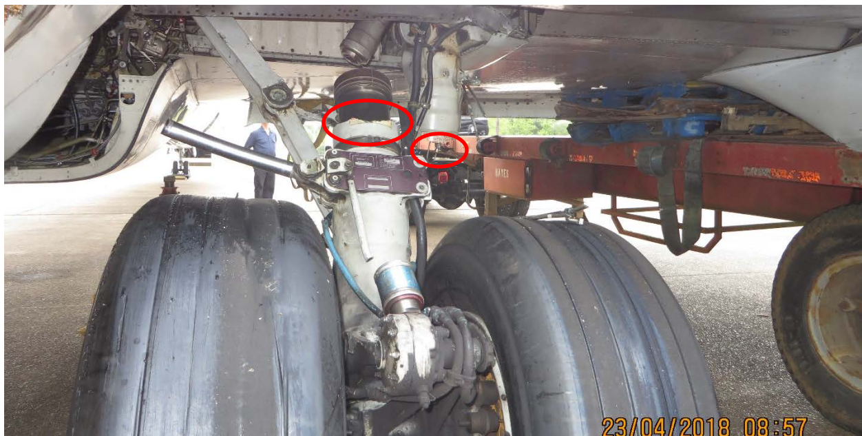
Figure 3 – Right main landing gear fracture looking forward.
