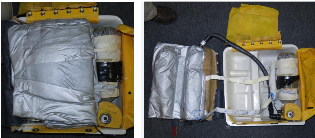
Figure 5 Slide Still in Packed Condition
