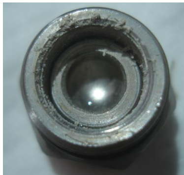
Figure 14 Internal Rupture Disk Intact
