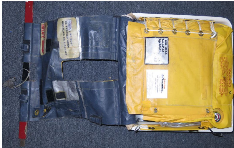
Figure 4 Slide System Prior to Inspection
